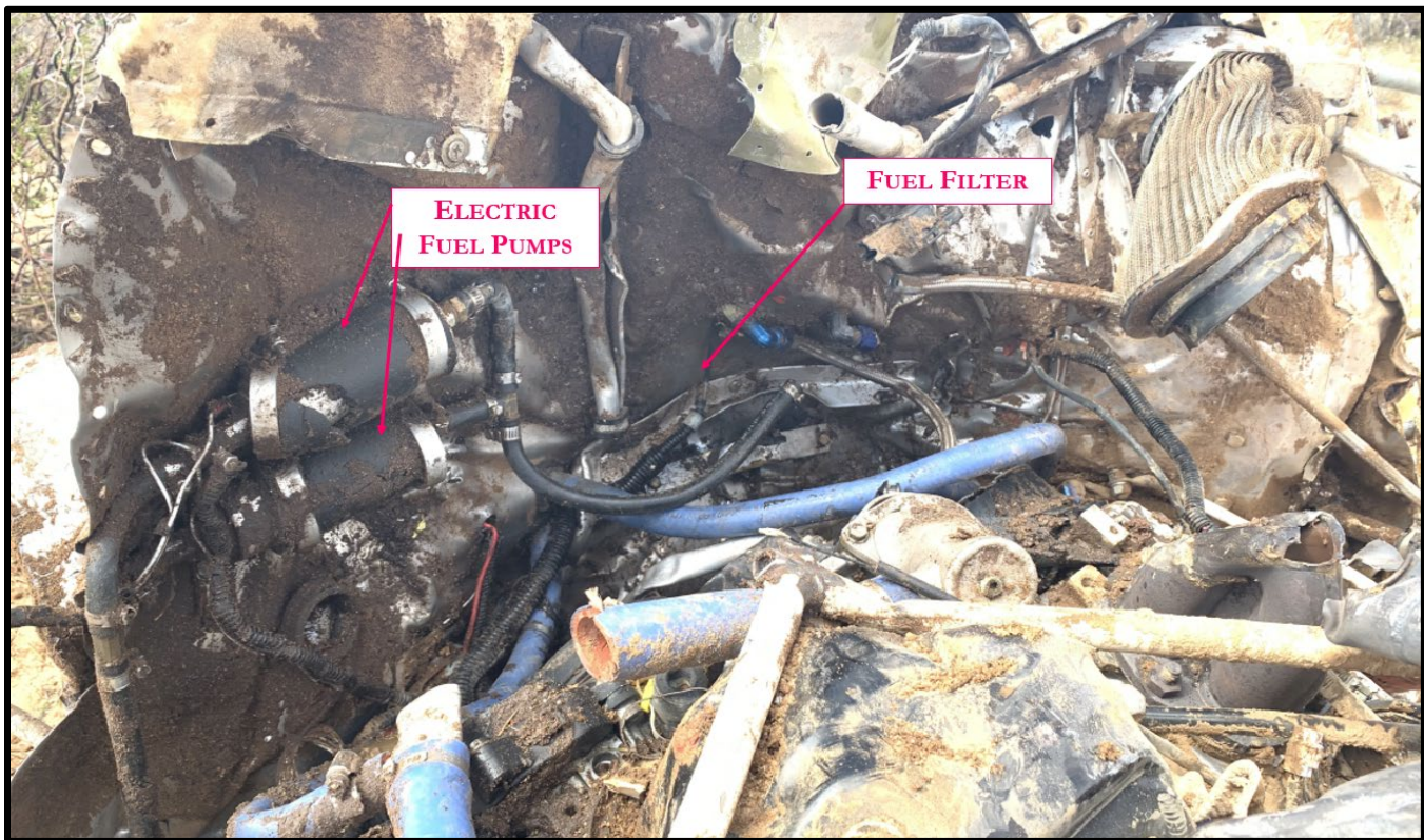
Figure 22: Fuel filters installed on the firewall.
