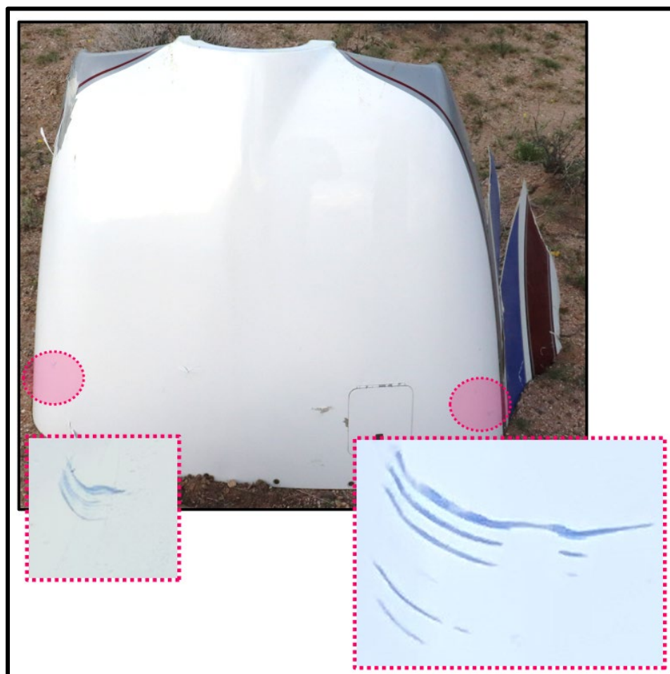
Figure 13: Marks on the top of the cowling.
