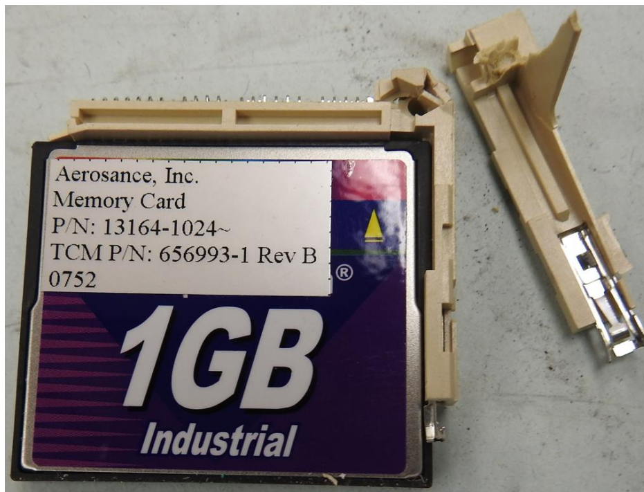
Figure 2. Recovered RDM CF memory card.
