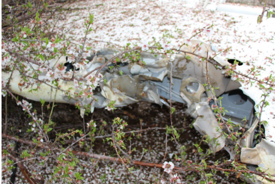
Photograph 3: Accordion style deformation at right wing
