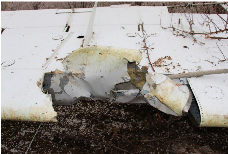
Photograph 4: Midspan damage at left wing with conductor
