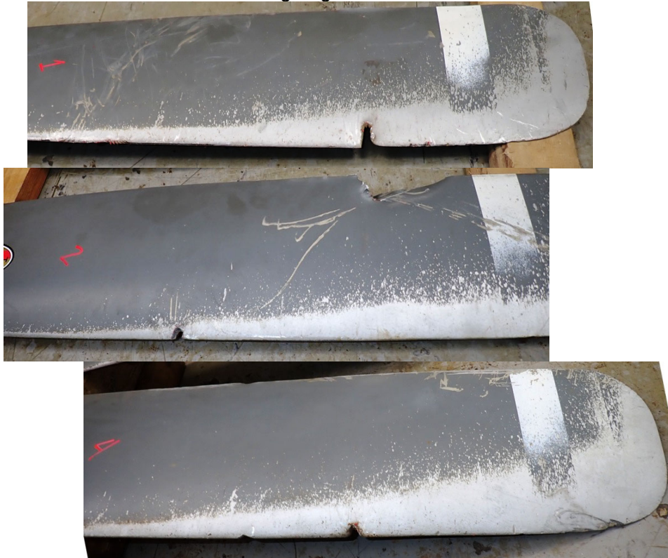
Photo #14 - Blade leading edge cable notch/cuts
