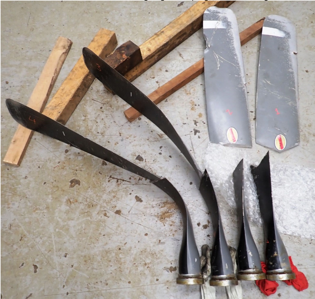
Photo #16 - Blades trailing edge view/progressive bending
