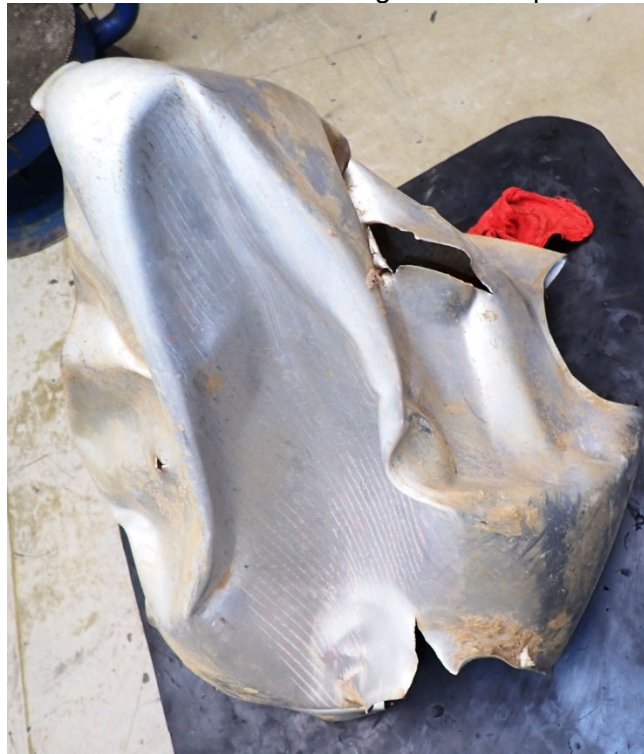
Photo #4 - Braided cable scoring marks in spinner dome
