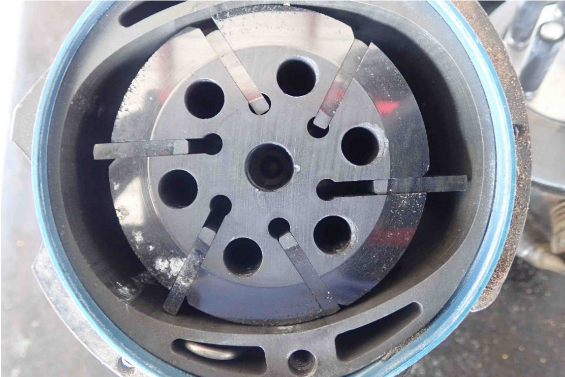
Figure 21 - Right Engine Vacuum Pump Vane and Blades
