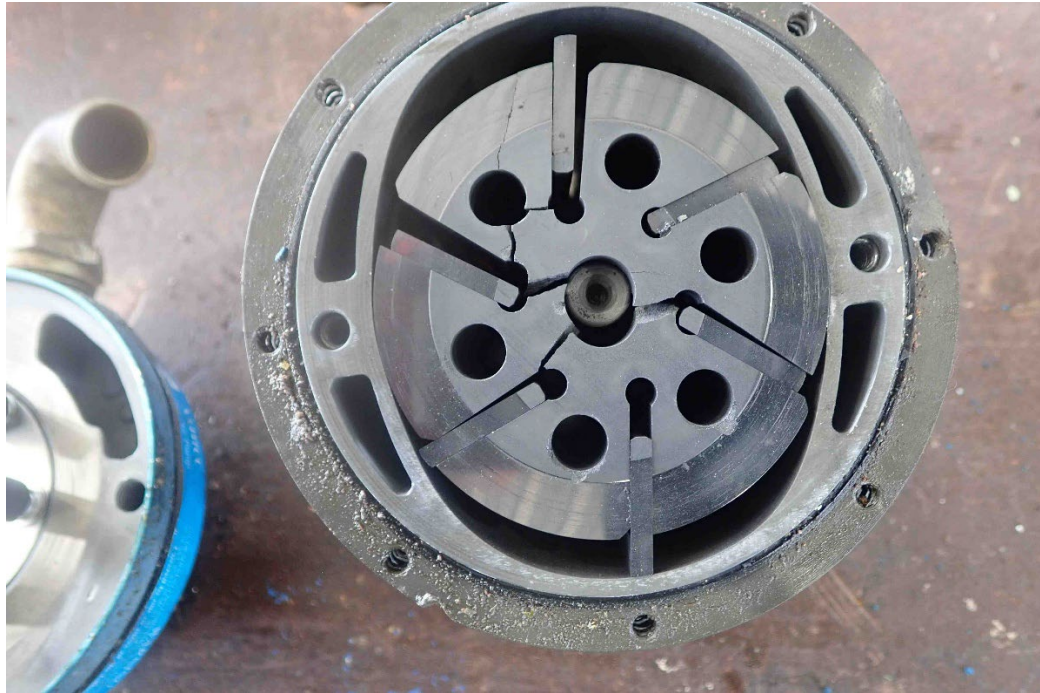
Figure 13 - Left Engine Vacuum Pump Vane and Blades
