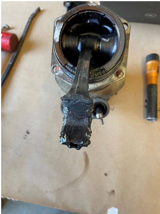
Figure 3: No. 1 piston rod and bearing failure
