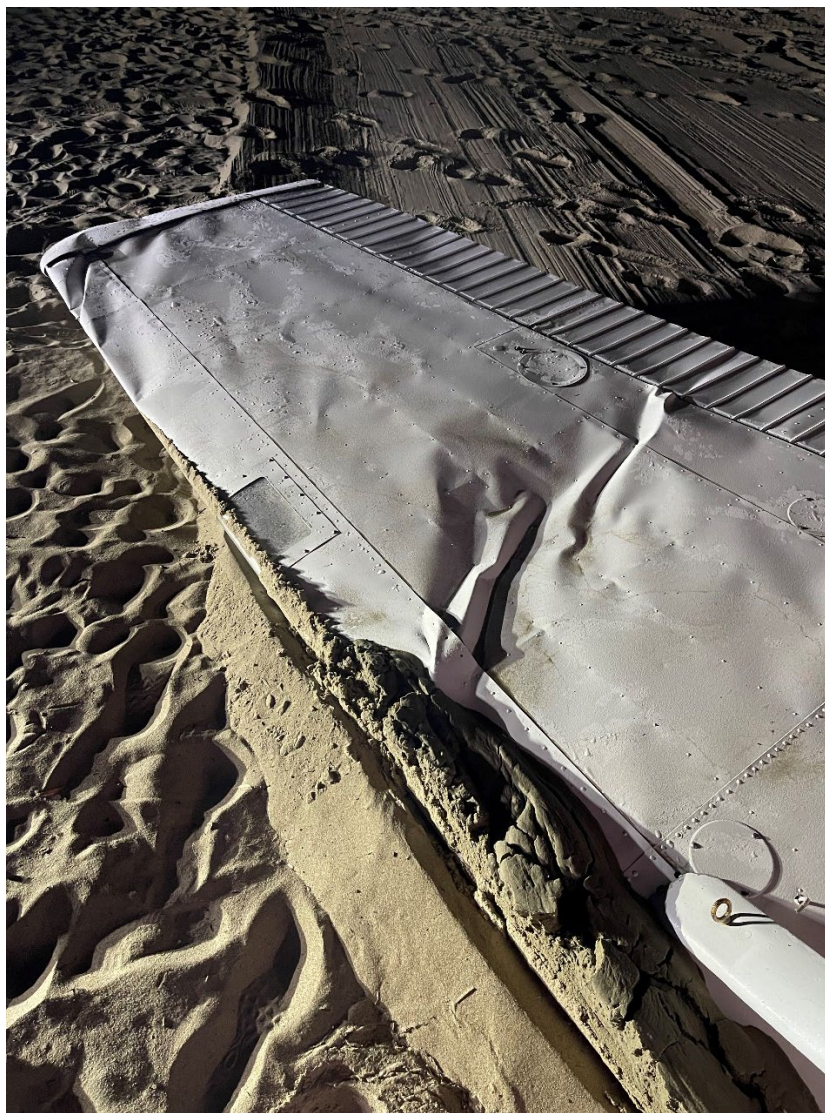
Photograph 3 - View of damage to left wing (Courtesy of LEO)
