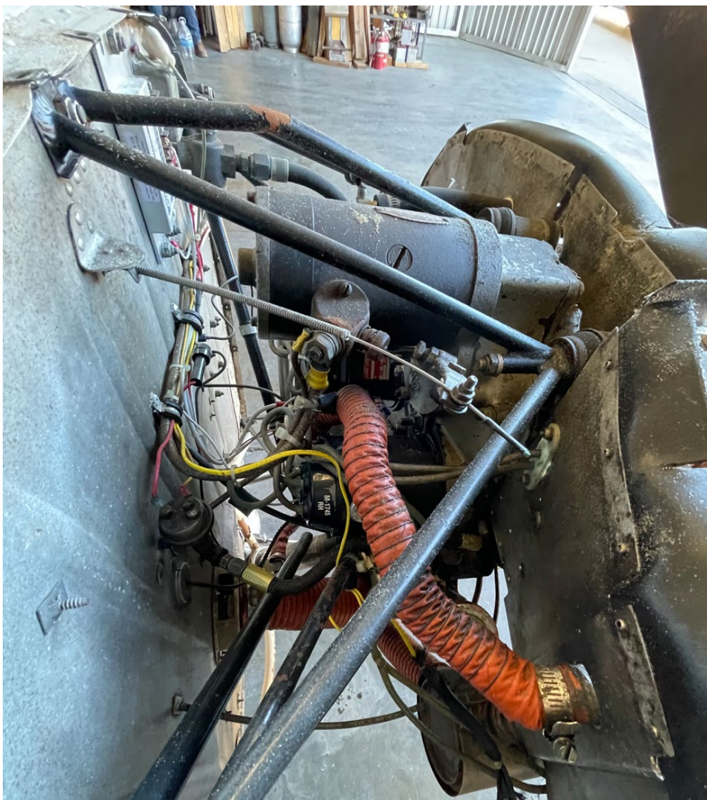
Photograph 5 - View of damage to upper and lower engine mounts (Courtesy of IIC)
