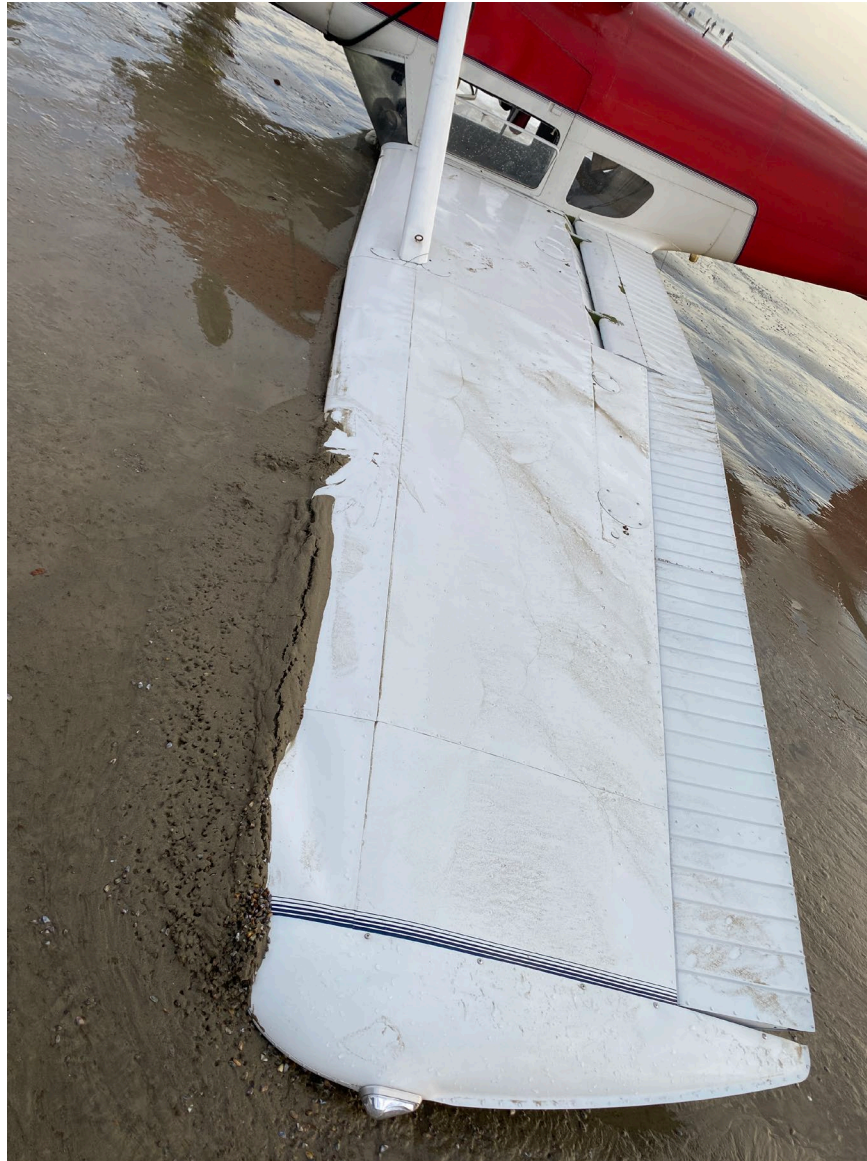
Photograph 4 - View of damage to the right wing (Courtesy of LEO)
