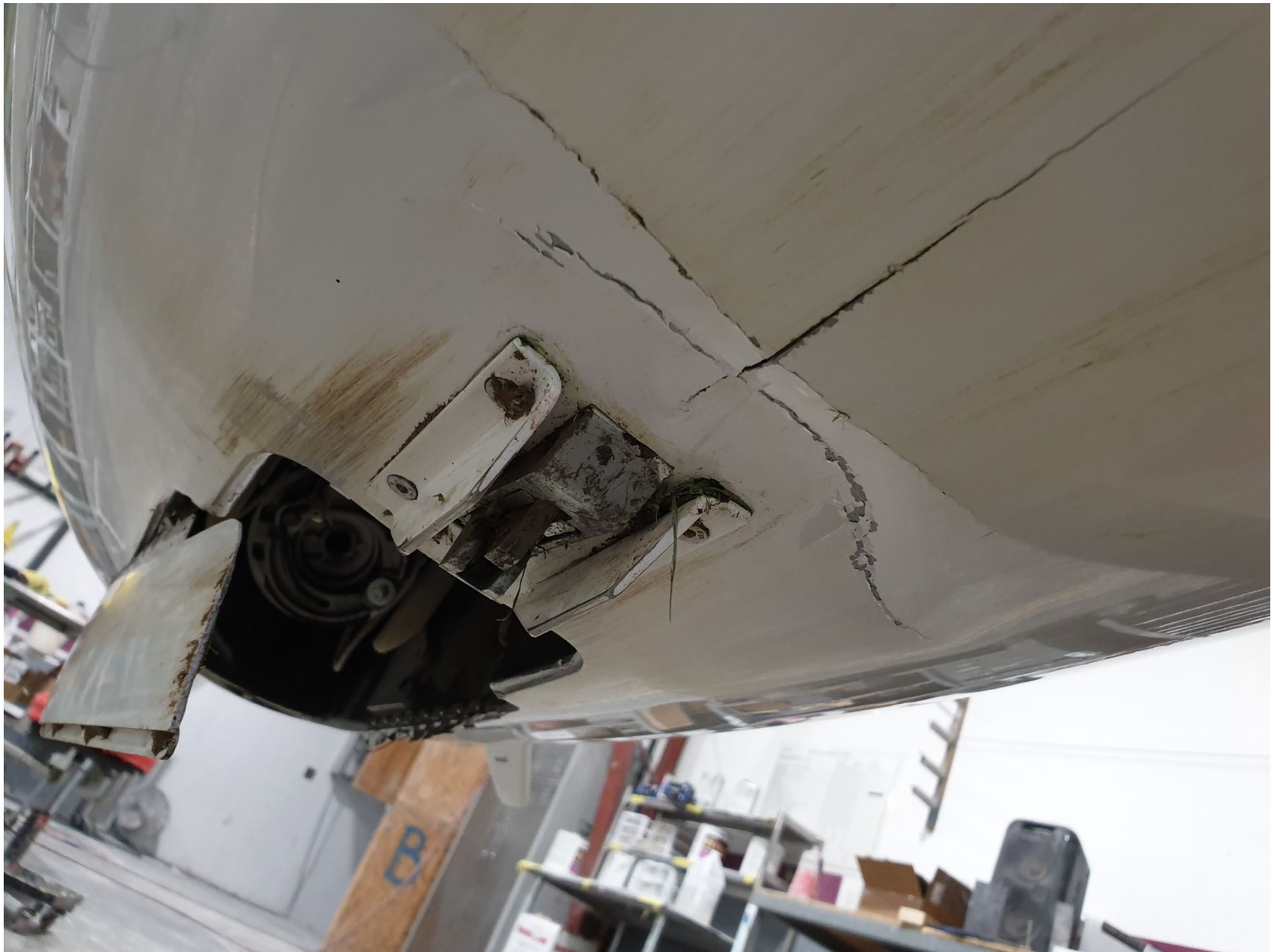
Photo 2 – View of Fuselage Damage (Courtesy of Pilot)
