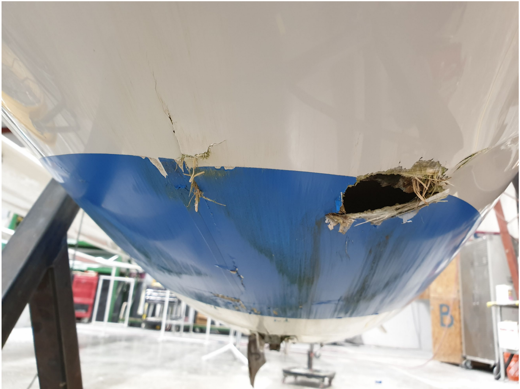
Photo 1 – View of Fuselage Damage (Courtesy of Pilot)
