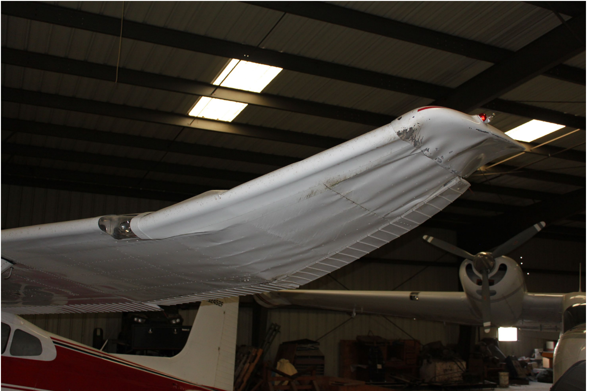
Photo 1 – View of Left Wing Damage (Courtesy of Pilot)
