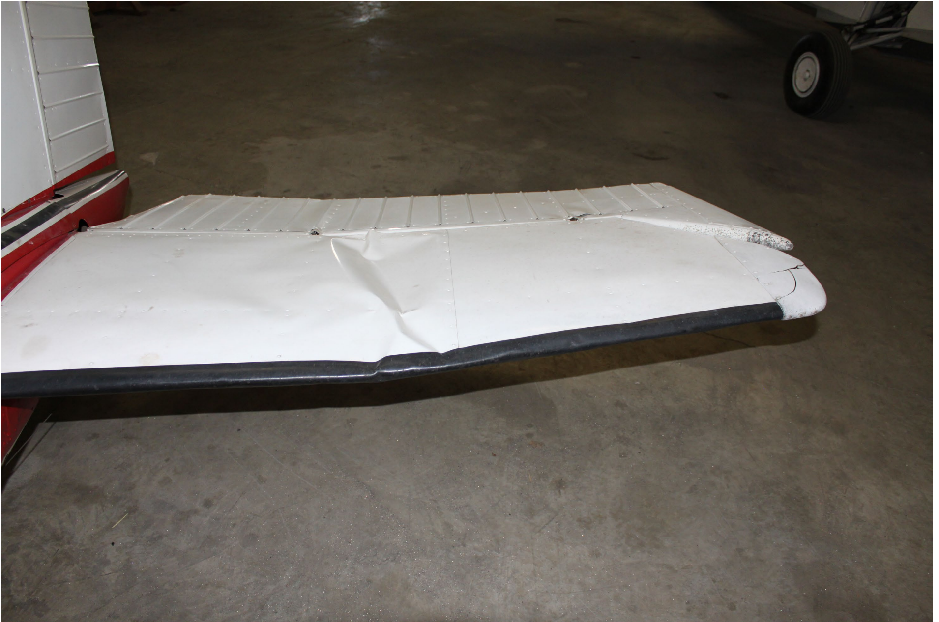
Photo 2 – View of Left Horizontal Stabilizer Damage (Courtesy of Pilot)
