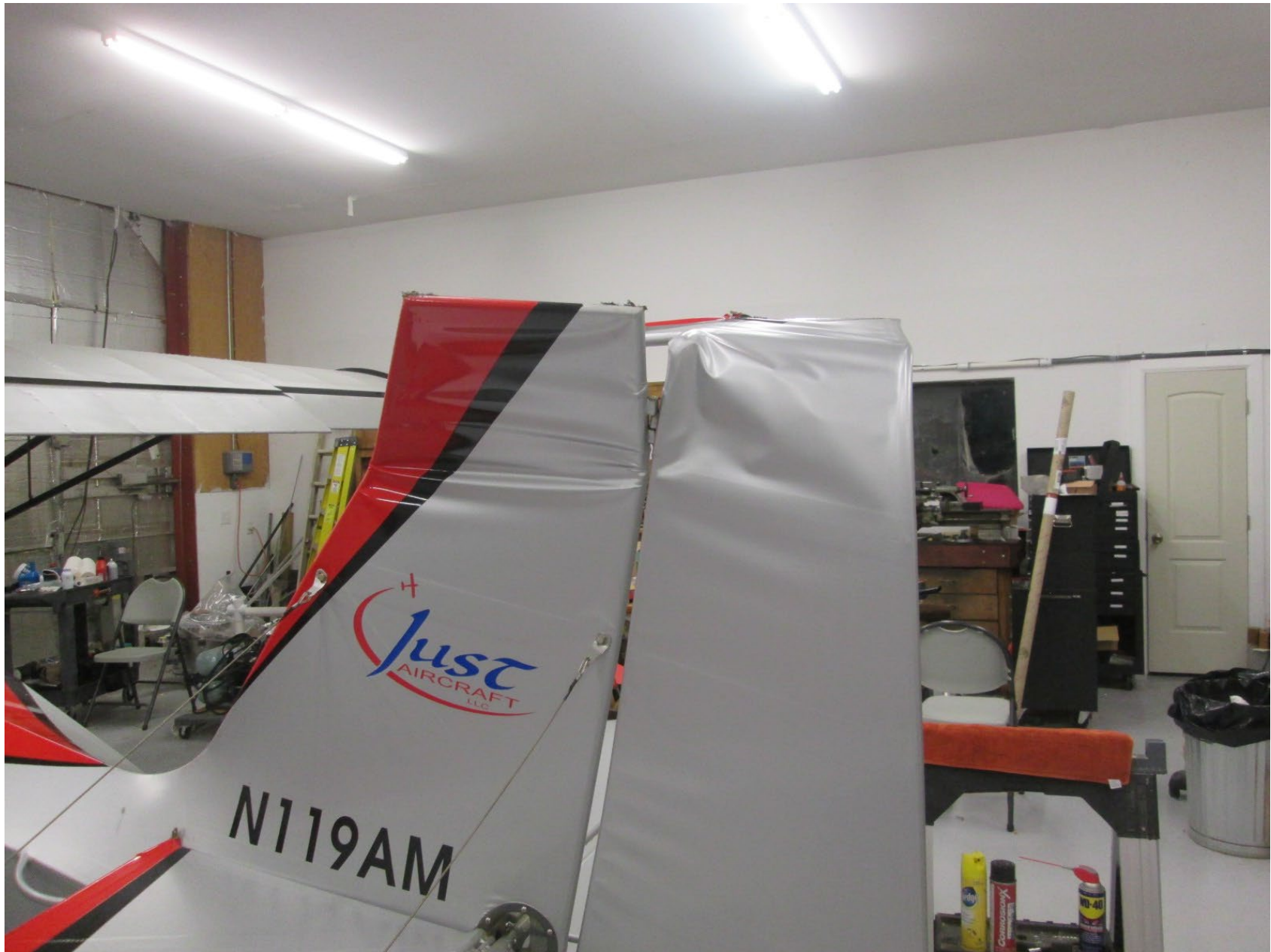
Photo 1 – View of tail damage (Photo courtesy of Tuolumne County Sheriff's Office)
