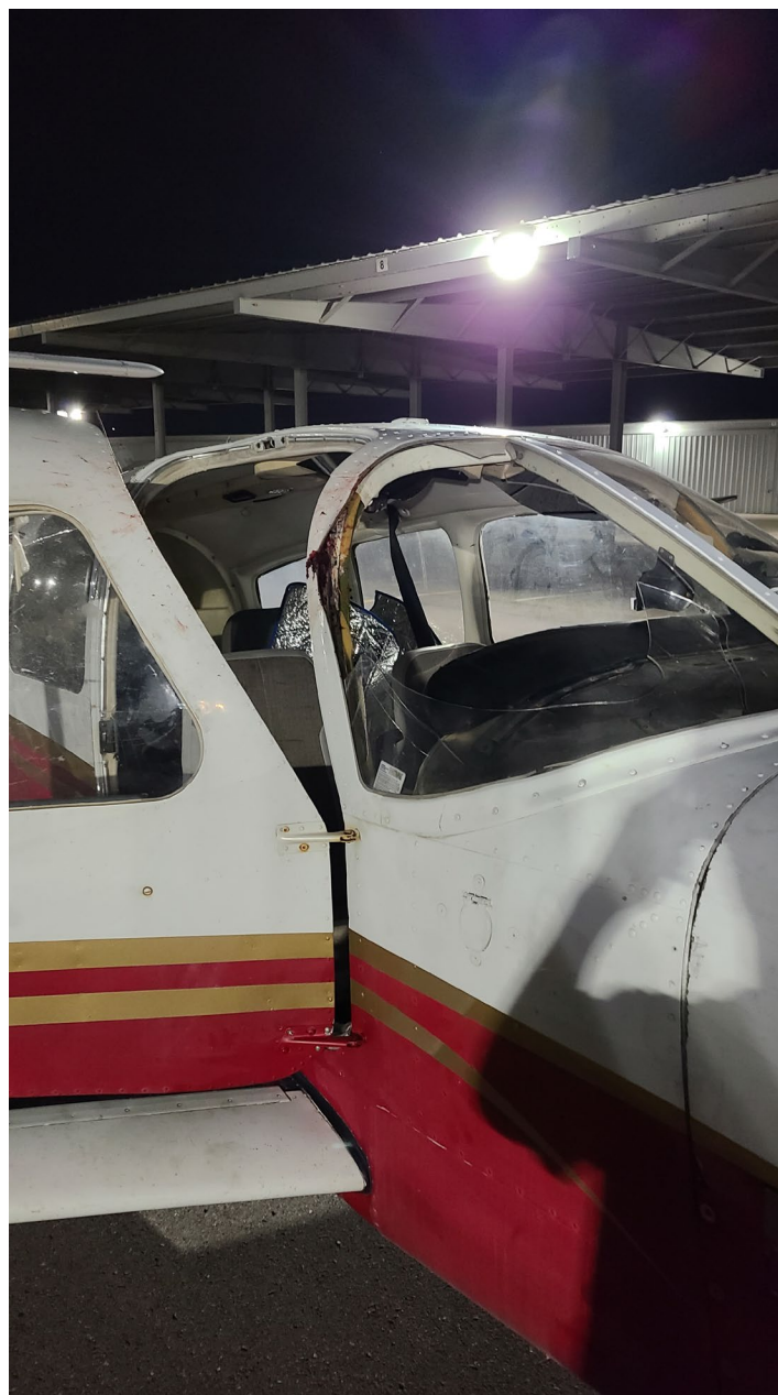
Photo 1 – View of substantial damage to windshield (photo courtesy of pilot)
