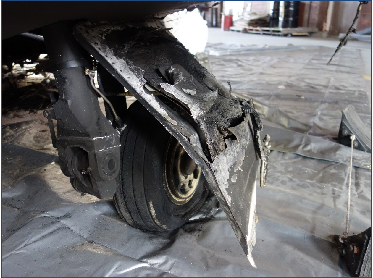
Photograph 4- The left main landing gear as viewed from the front.
