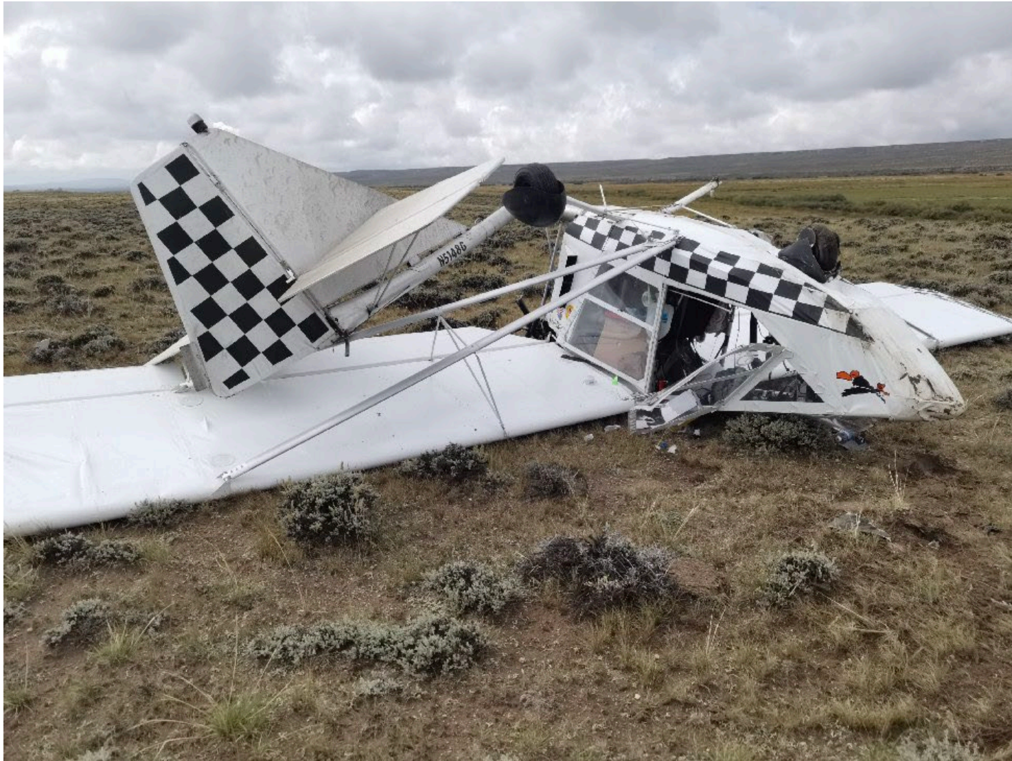
Photograph 1 - View of nosed over airplane in an open field with damage to tailcone and wings (Courtesy of Highway Patrol Supervisor)
