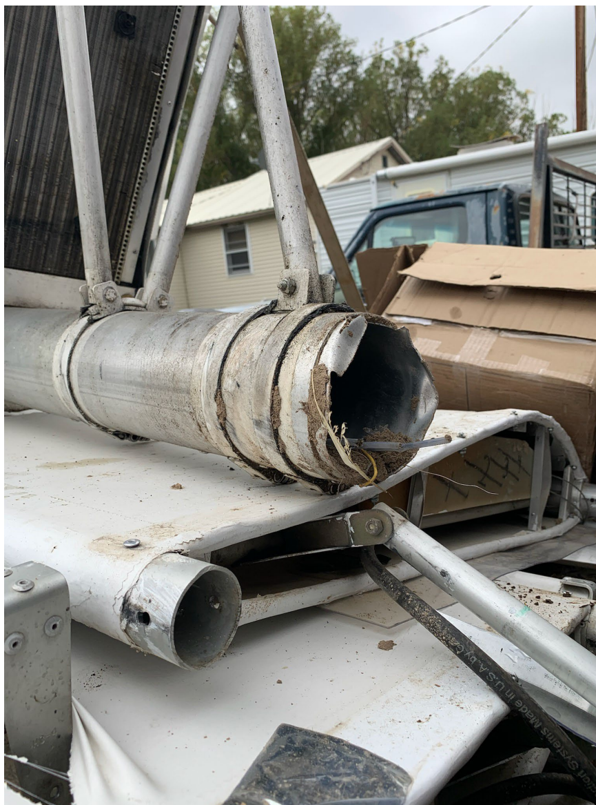
Photograph 5 - View of damaged tailcone (Courtesy of FAA Inspector)
