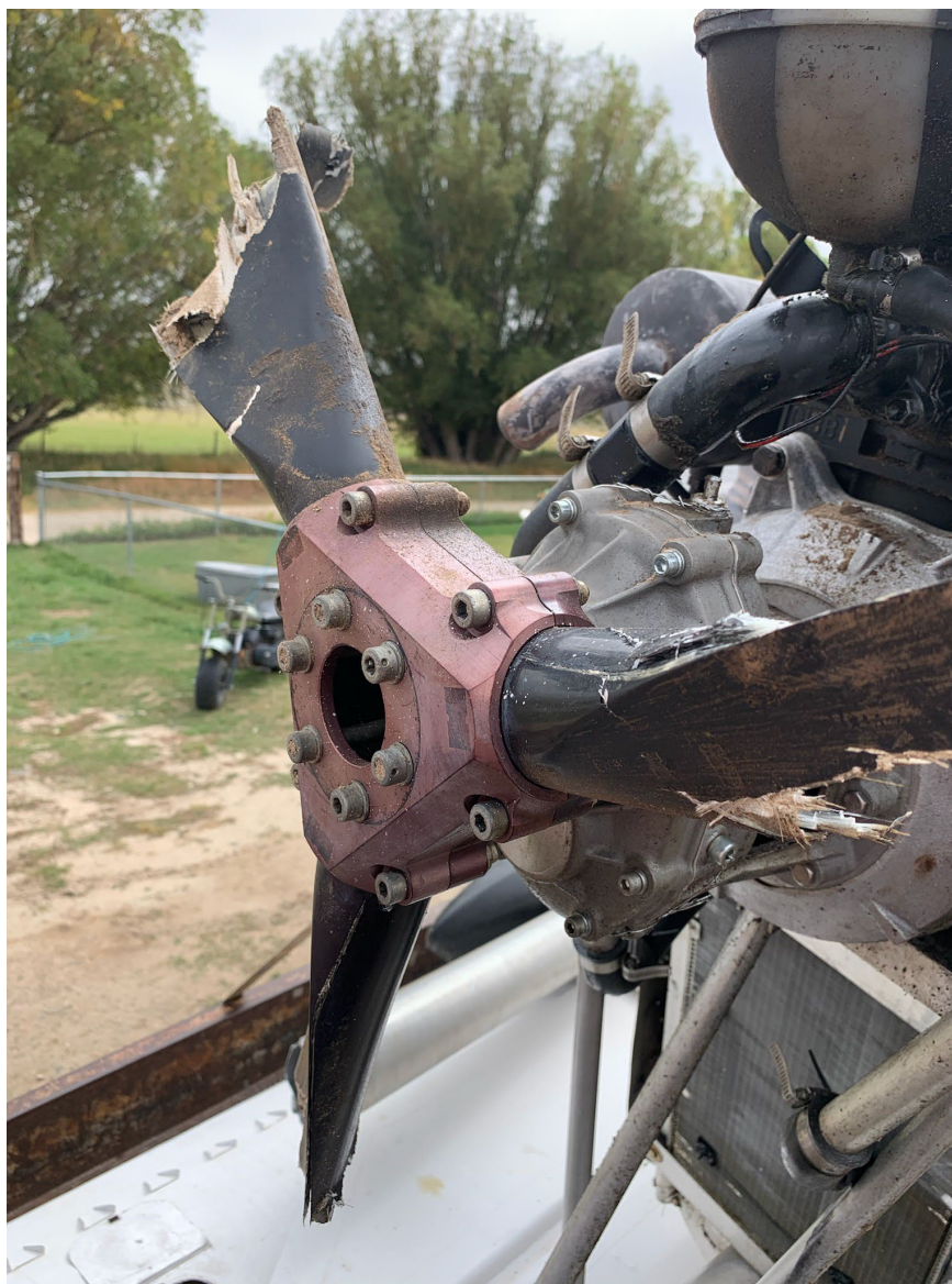
Photograph 4 - View of damaged 3-bladed propeller (Courtesy of FAA Inspector)
