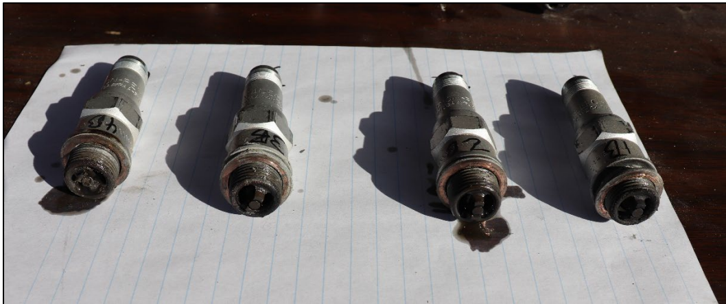
Figure 10: View of bottom engine spark plugs
