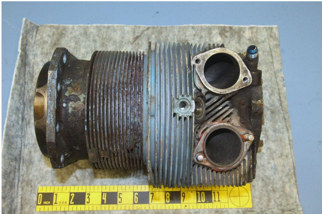
Figure 1. View of the cylinder from the side with the intake and exhaust ports.
