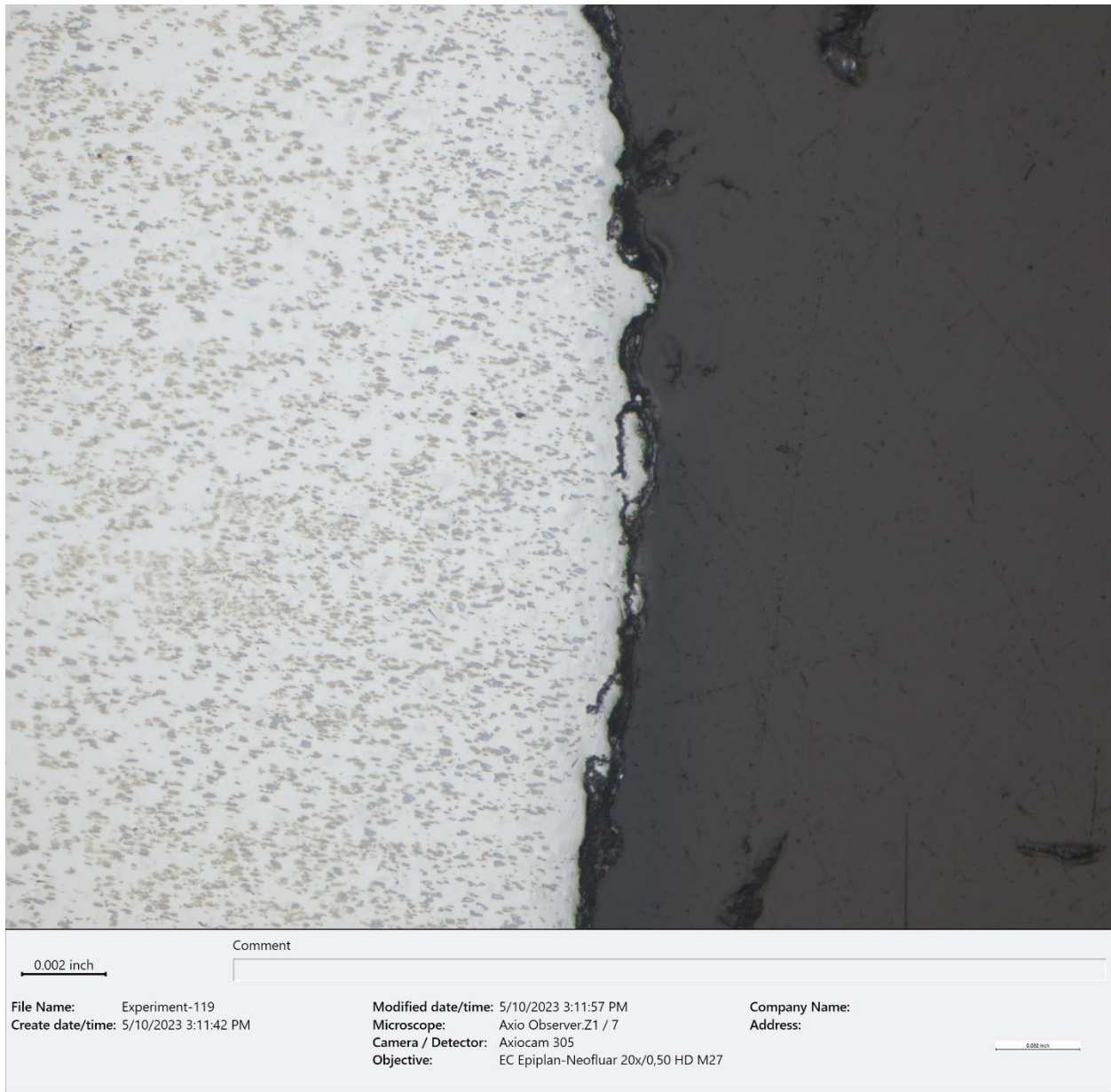
Figure 22. BF optical micrograph of small internal secondary cracks along the fracture surface (~200X, as polished).
