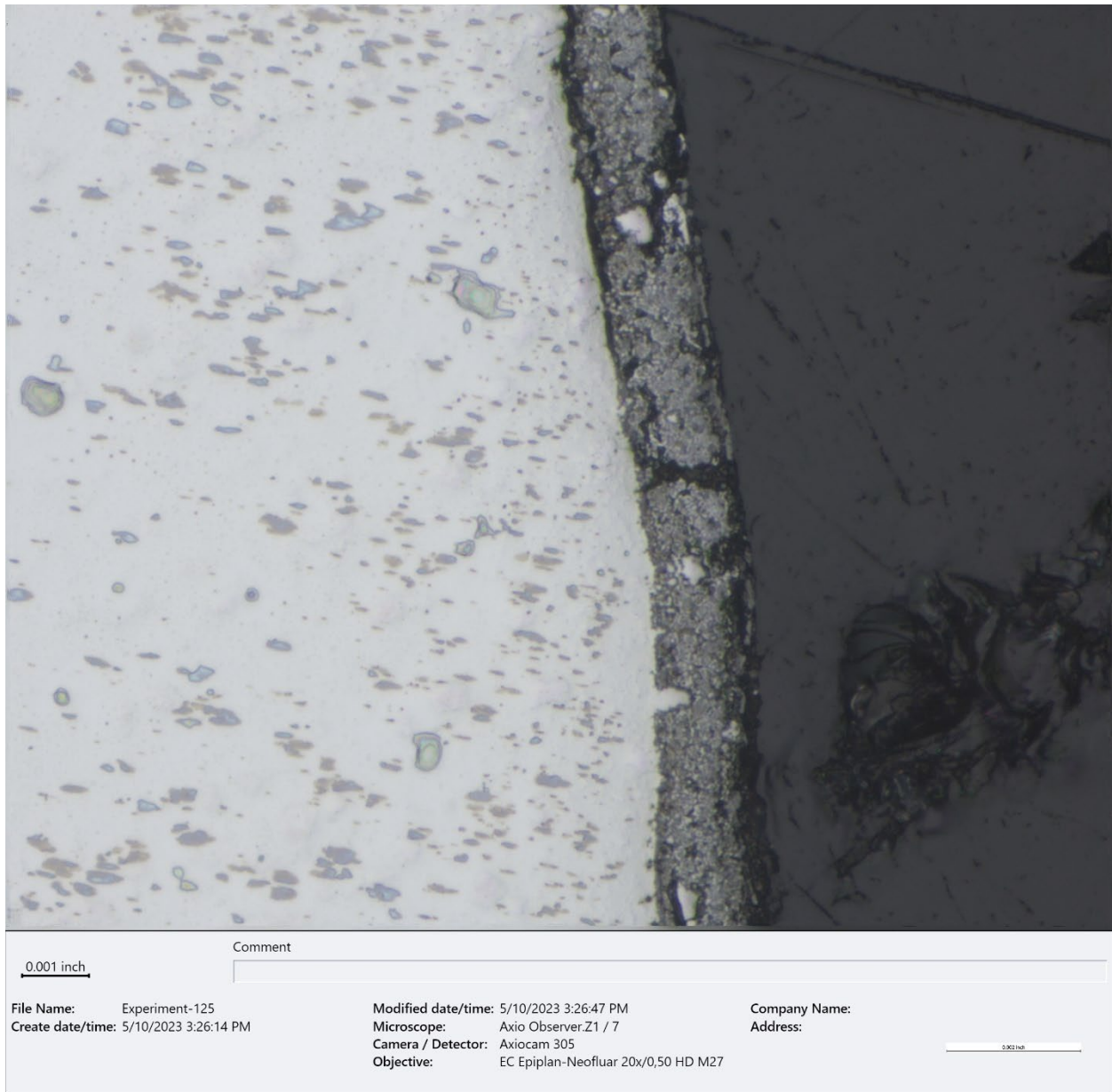
Figure 20. BF optical micrograph of nonmetallic deposits on the fracture surface of the fractured valve stem (~500X, as polished).
