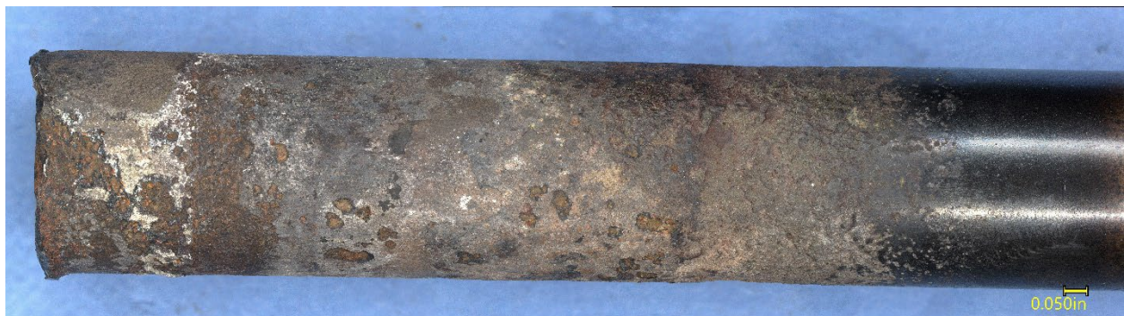
Figure 7. Side view of the exhaust valve stem remnant, after cleaning.
