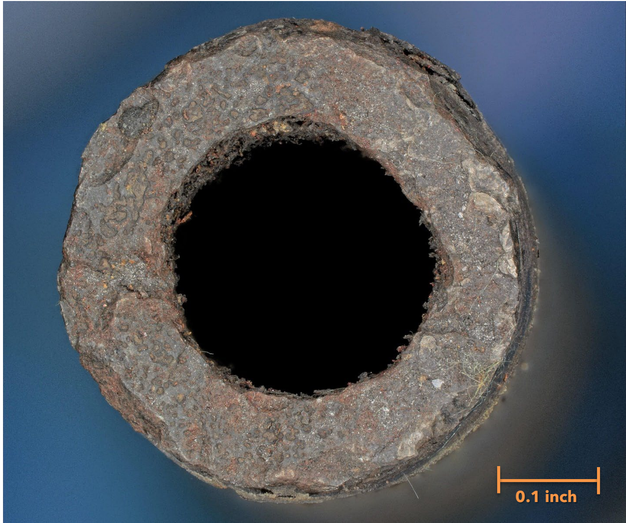
Figure 5. View of the exhaust valve stem fracture surface after degreasing.
