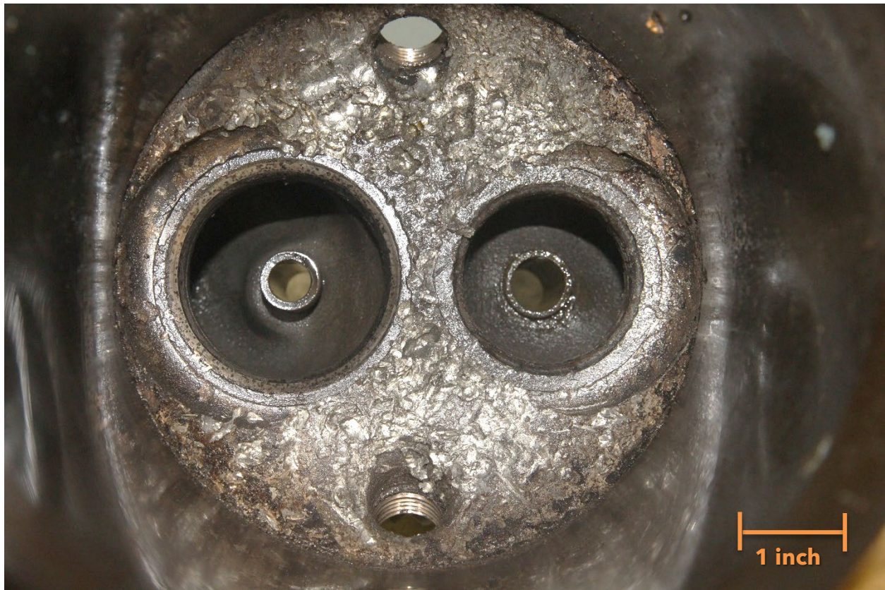
Figure 3. Closer view of the interior of the cylinder, showing impact damage to the cylinder and valve seat surfaces.
