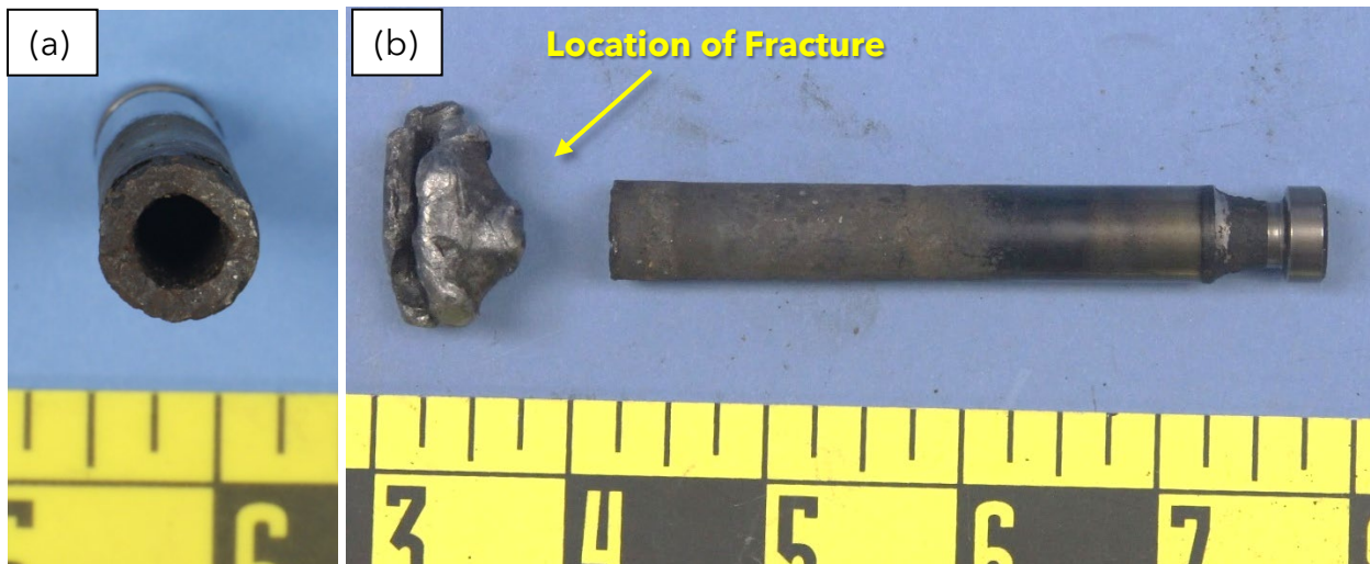
Figure 4. View of the fractured exhaust valve from (a) the stem fracture and (b) side showing the stem side and liberated valve head remnant.
