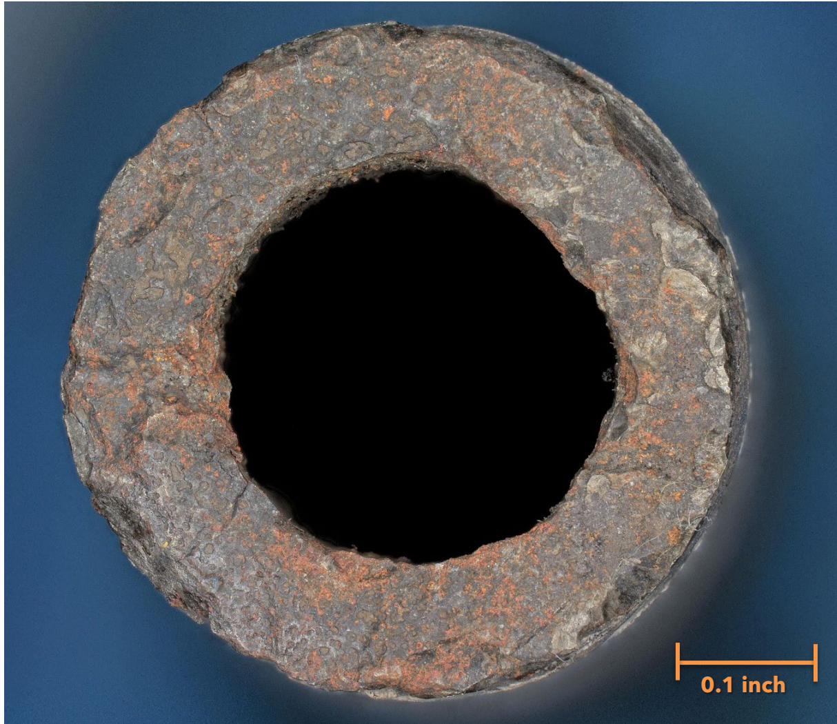
Figure 6. View of the exhaust valve stem fracture surface after cleaning with Evaporust.
