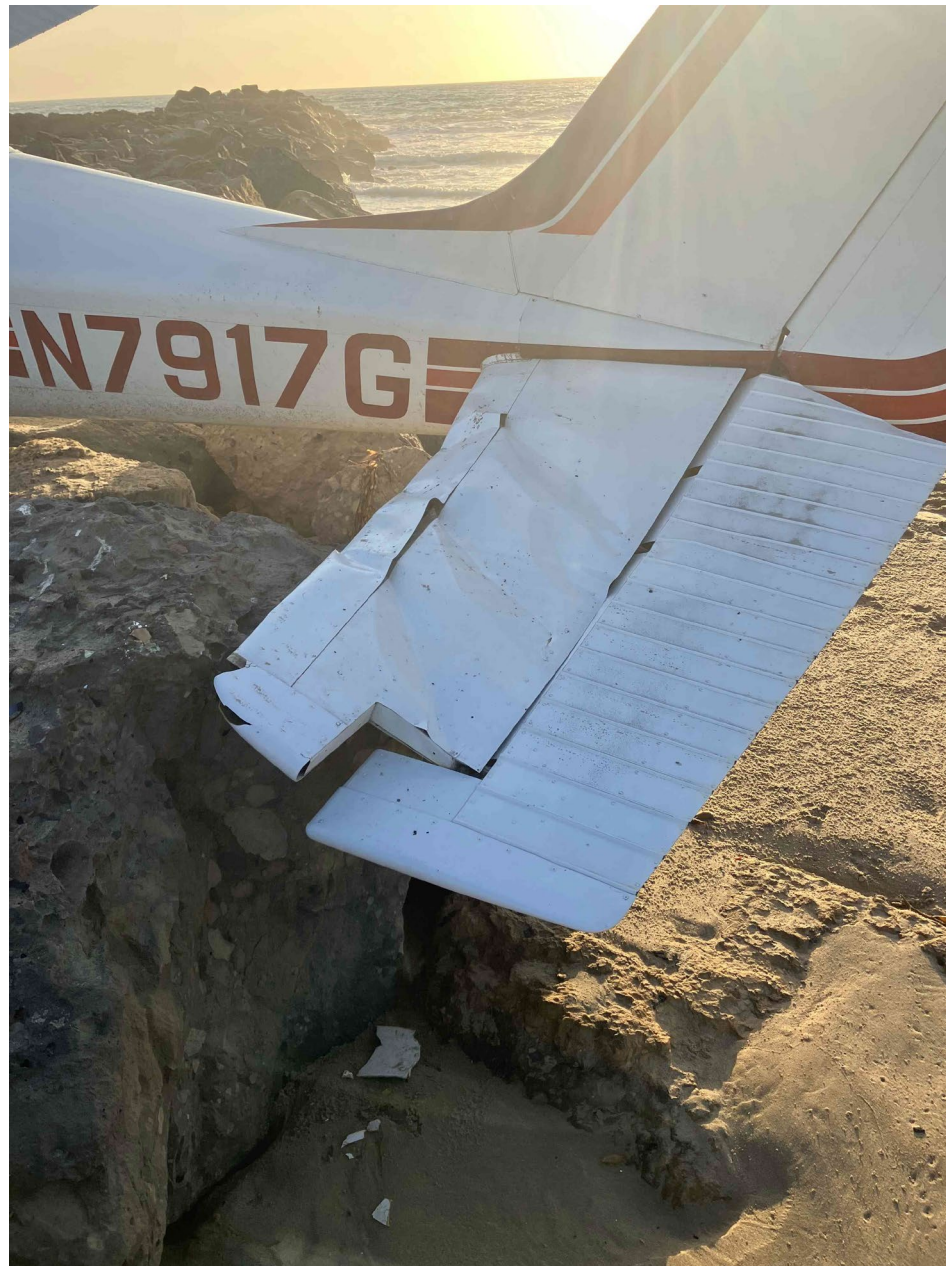
Photo 3 – View of left Horizontal Stabilizer damage (photo courtesy of Airport Operations)
