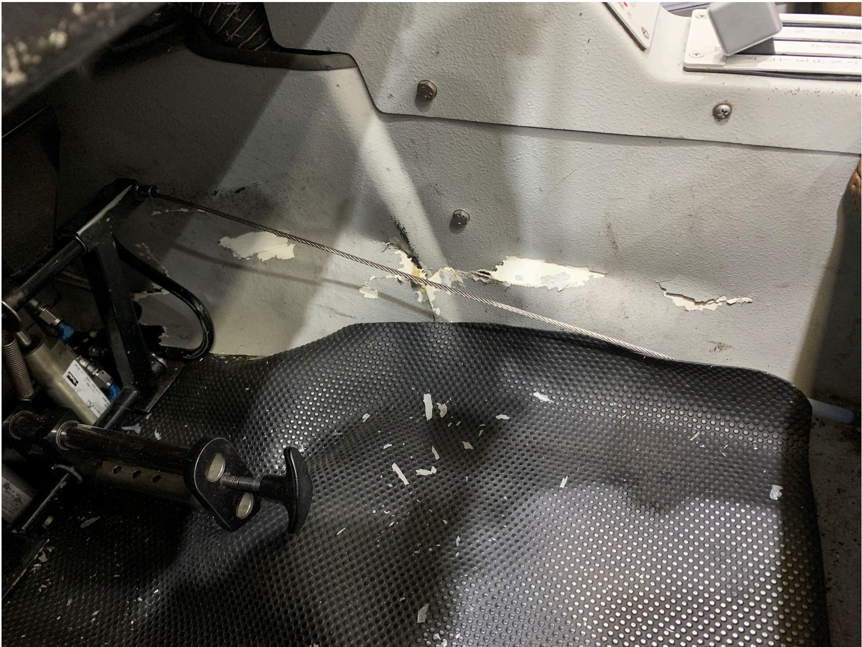
Photo 1 – View of pilot side center pedestal / floorboard damage (Photo courtesy of Clark County DOA)
