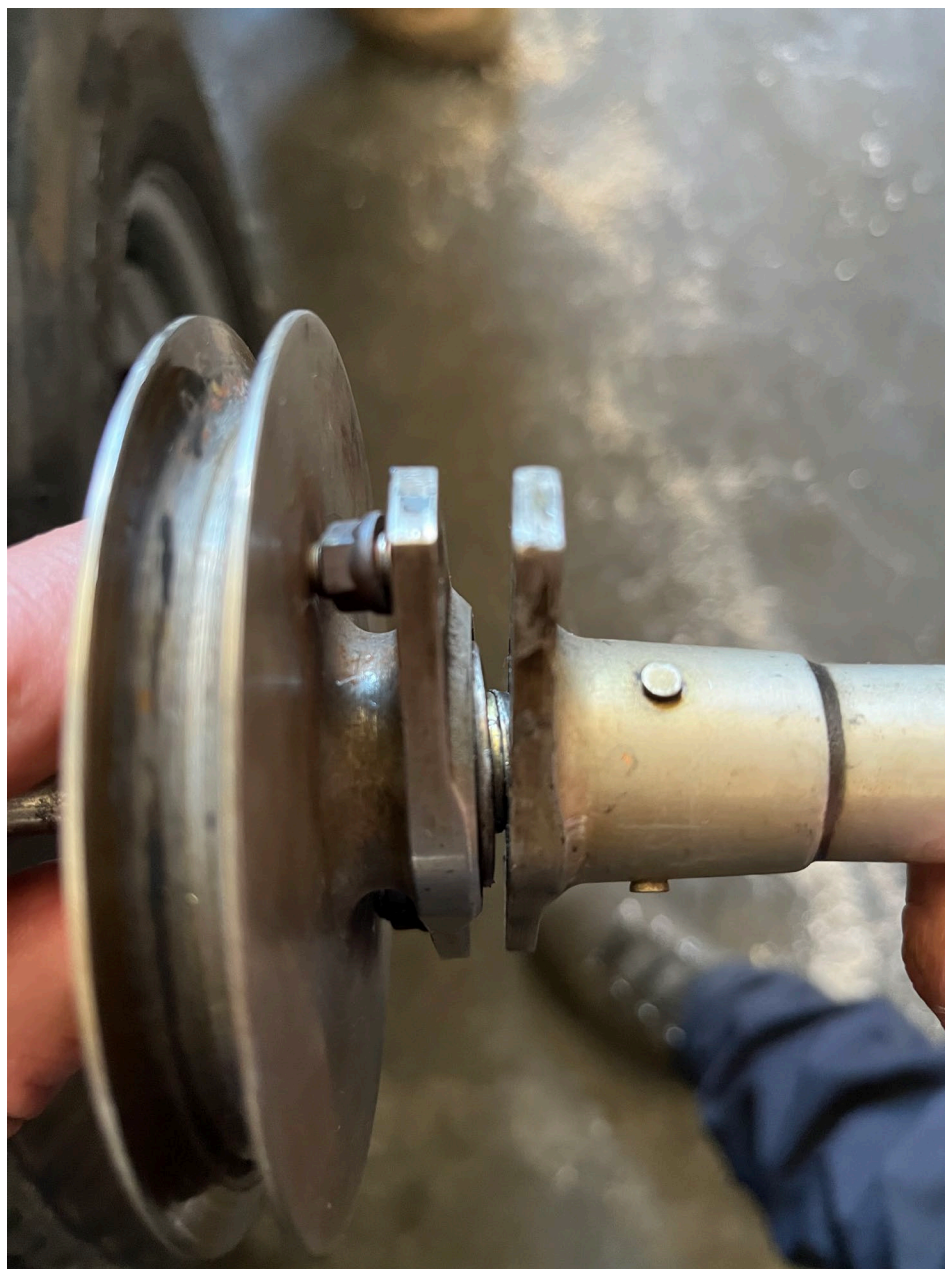
Photo 5 – Air conditioning pulley with bolt and nuts trapped in the holes. Photo courtesy of Cal-Fire.
