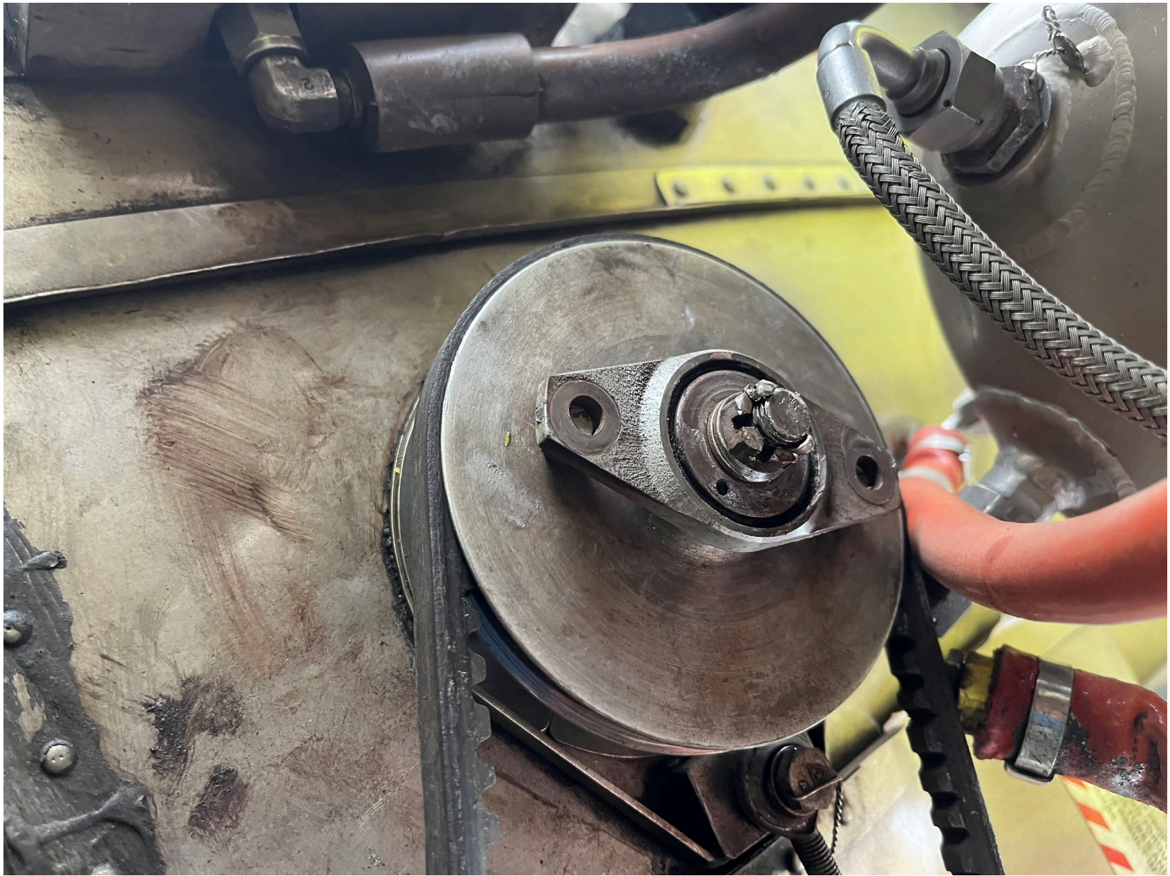
Photo 4. Air conditioning pulley with tail rotor drive shaft attachment flange. Photo courtesy of Cal-Fire
