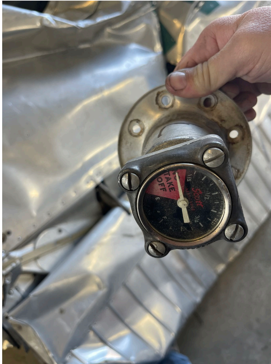
Photograph 4 - View of one of the removed fuel gauges.
