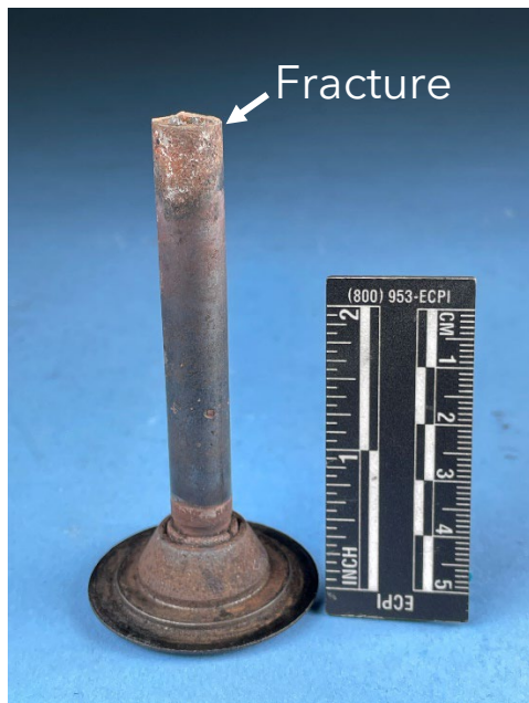
Figure 2. Side view of the fractured valve stem, after cleaning.
