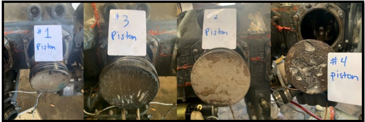
Figure 6. View of piston faces with mechanical damage to piston no. 4 (4 total view)
