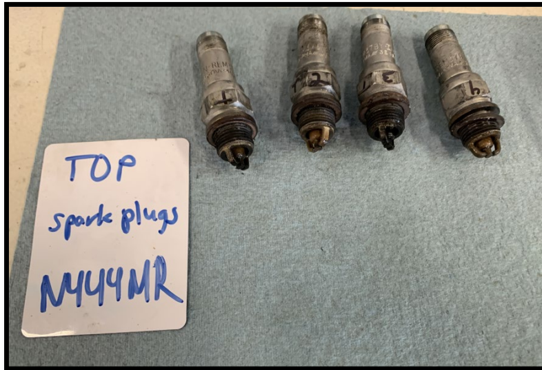
Figure 4. View of all top spark plugs from accident engine
