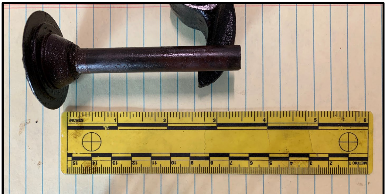
Figure 9. View of No. 4 cylinder exhaust valve measurement
