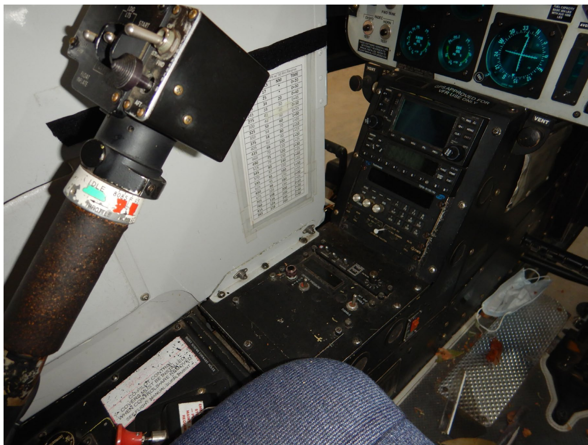
Photograph 2 - Collective Grip Twist Throttle Installed (Courtesy of NTSB)
