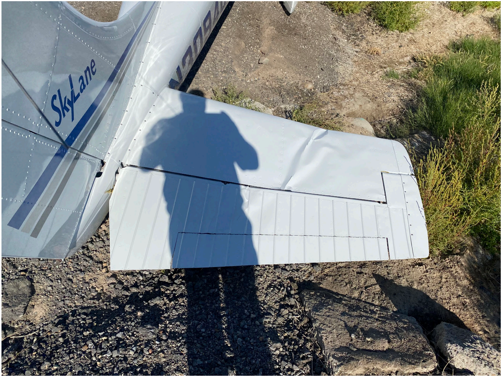
Photo 2 – View of right horizontal stabilizer and elevator damage (photo courtesy of airport operations)
