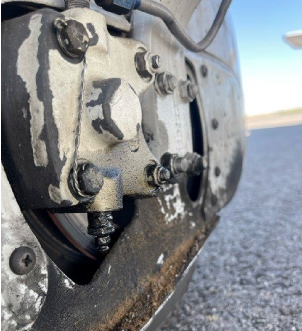
Figure 2: View of right main landing gear brake caliper (photo courtesy of A&P)
