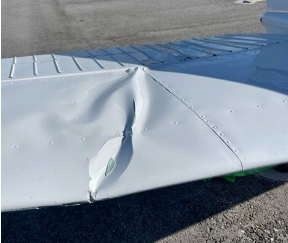
Figure 1: View of right horizontal stabilizer and elevator damage (photo courtesy of A&P)
