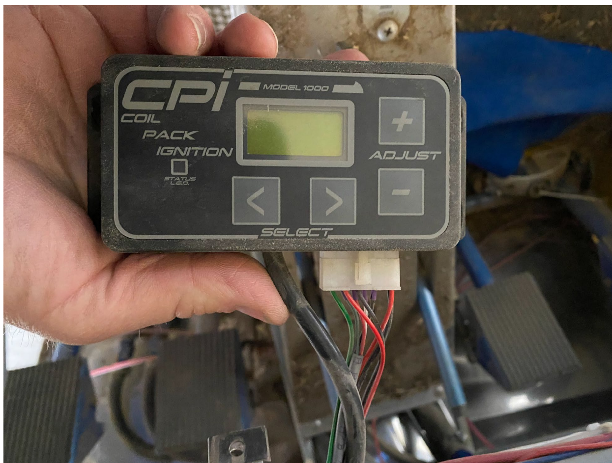
Figure 1. Coil Pack Ignition, Model 1000 (Photo courtesy of the FAA)
