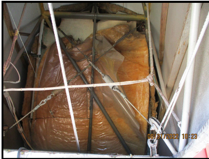
Figure 1: Interconnect between the aileron and the rudder (Source: FAA)
