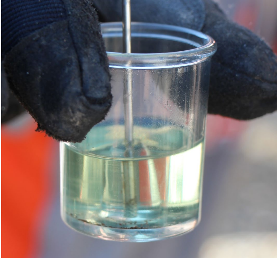
Photograph 2: Sample from fuel strainer bowl
