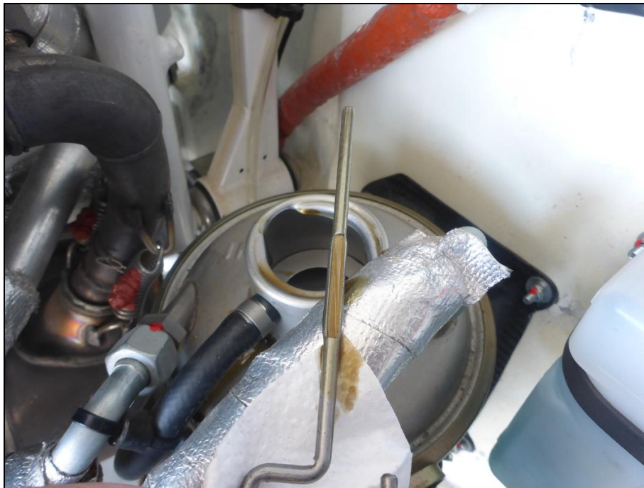
Figure 6-Oil tank dip stick.
