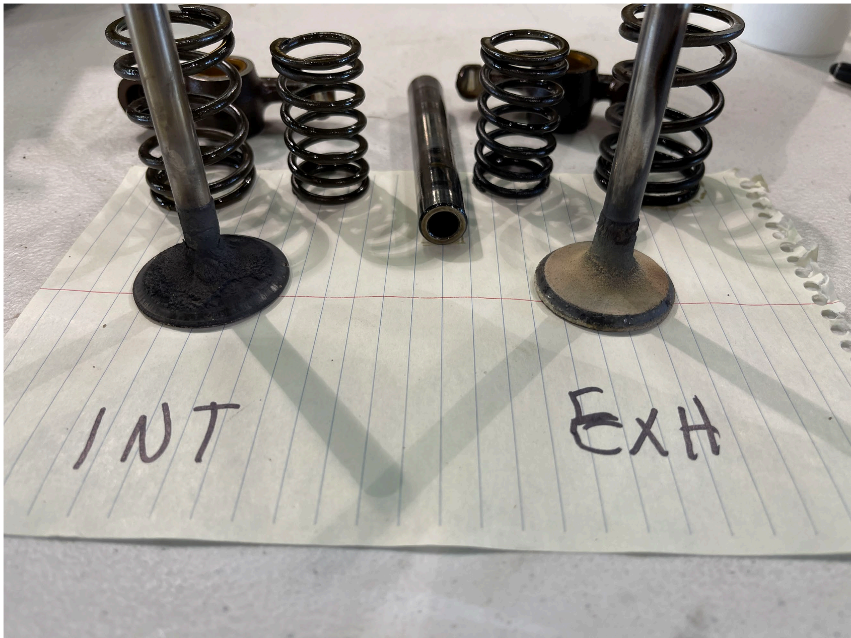
Photo 5 – No. 2 Cylinder Intake and Exhaust Valves
