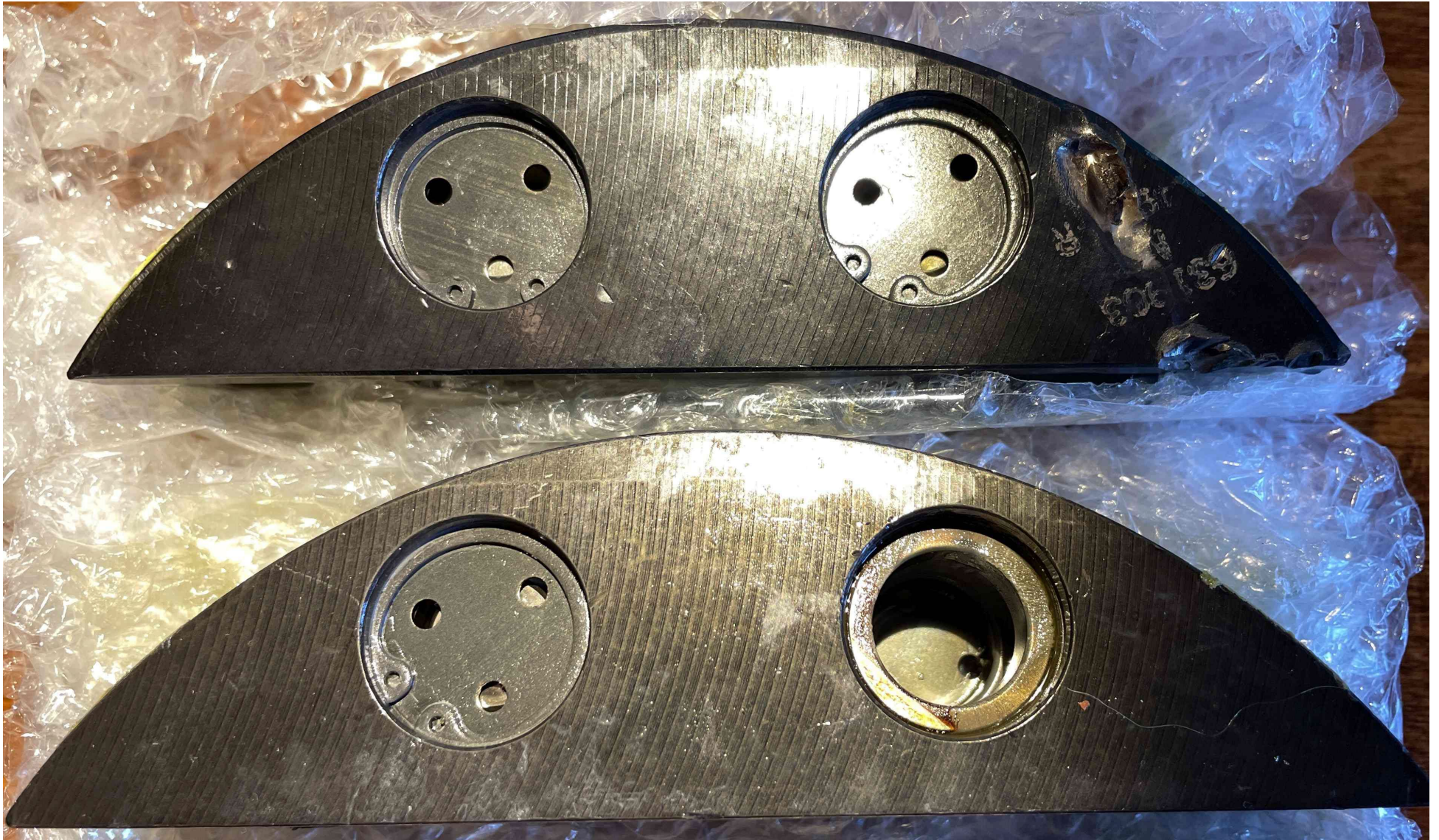
Photo 1 – Cylinder number 1 and 2 counterweight with two incorrectly installed retaining clips (top right, bottom left).
