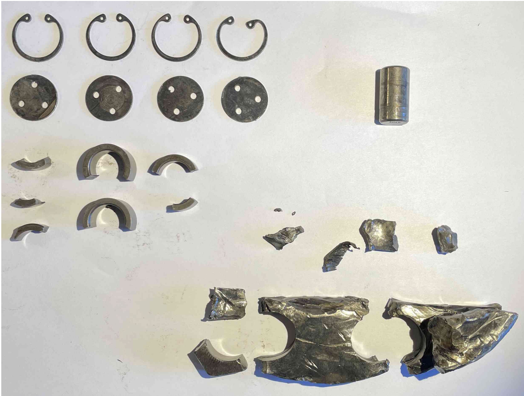
Photo 3 – Fragments of counterweight, bushings, a single counterweight pin, and four retaining rings and plates
