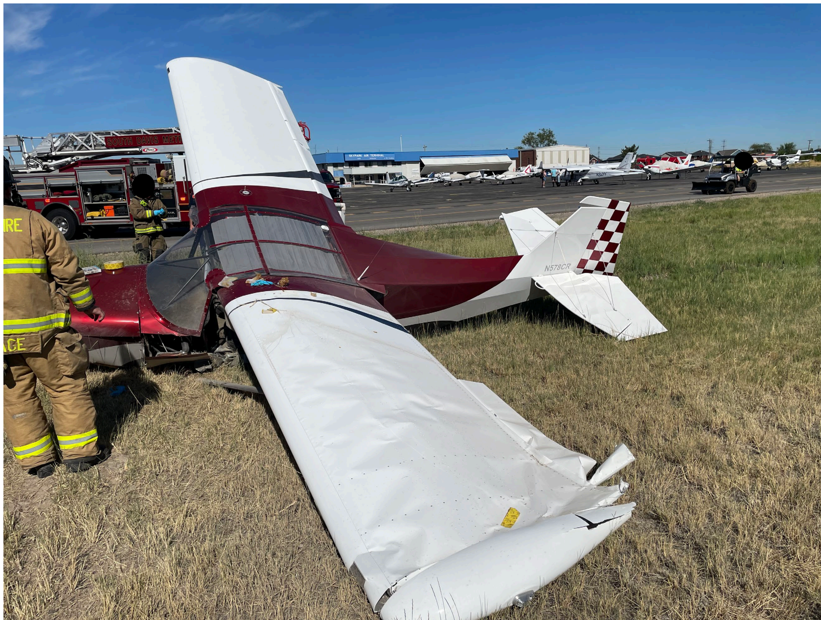
Photo 1 – View of Damage to Left Wing and Fuselage (Courtesy of FAA)
