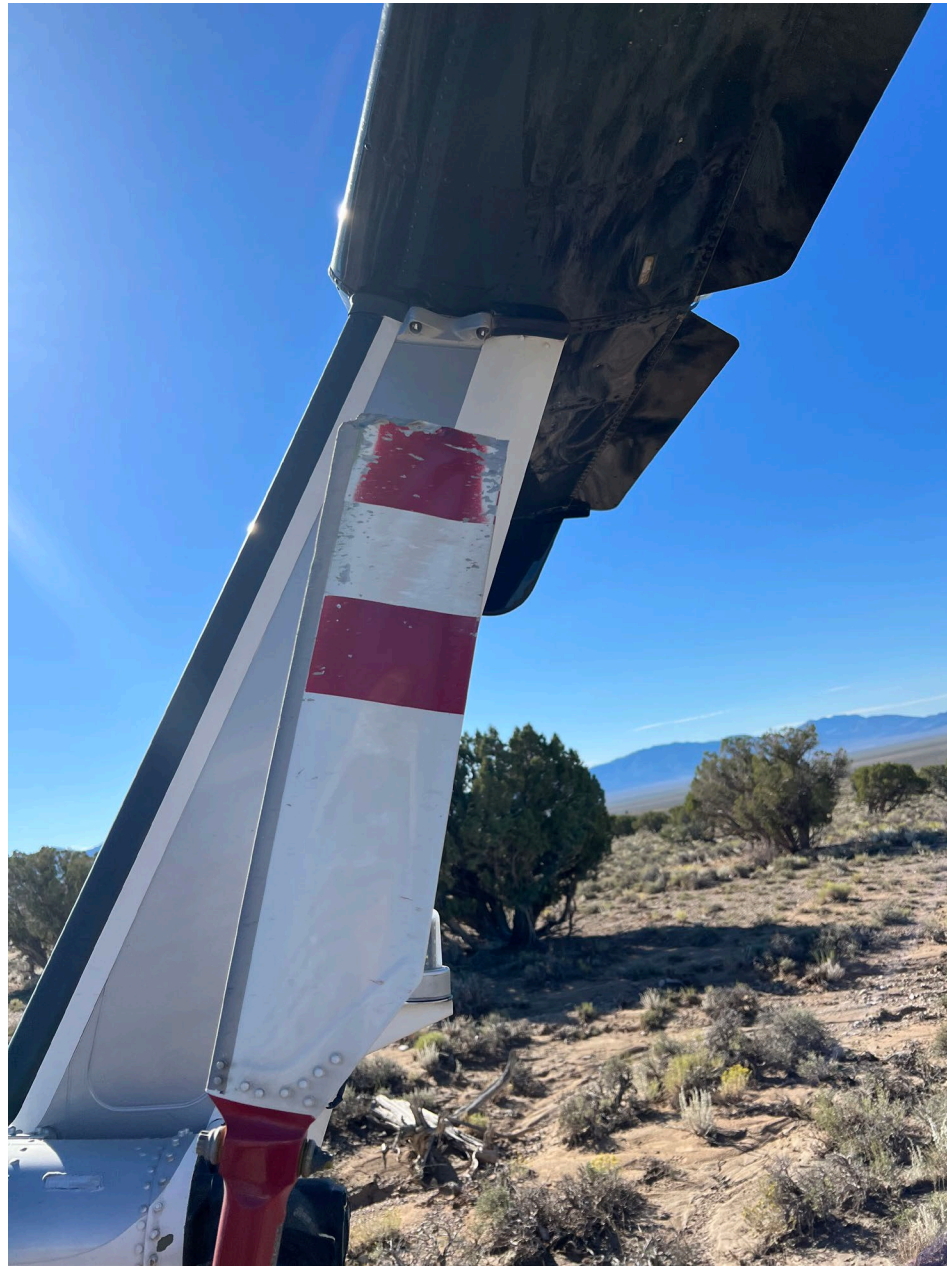
Photo 1 – Rotor damage of sheared tail rotor shaft
