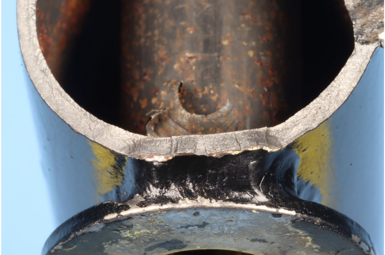
Figure 4. Fracture surface 2 exhibiting a thumbnail shaped fatigue crack and ratchet marks.
