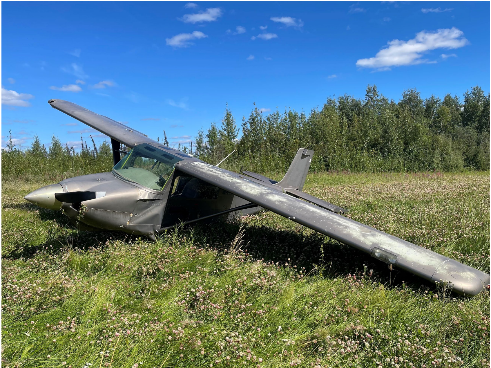
Photo 1 – View of forward fuselage damage (photo courtesy of the pilot)
