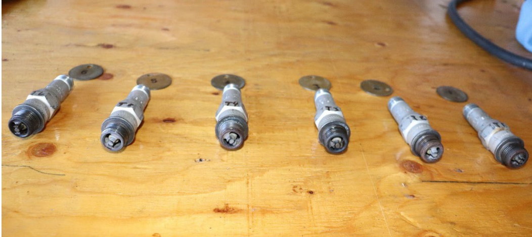
Figure 8: View of top engine spark plugs
