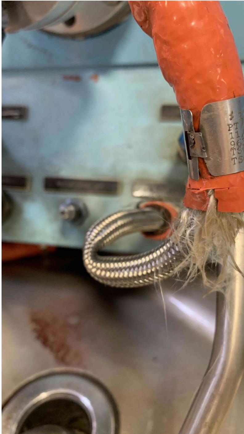
Figure 10 - Output line twisted until flow limited
