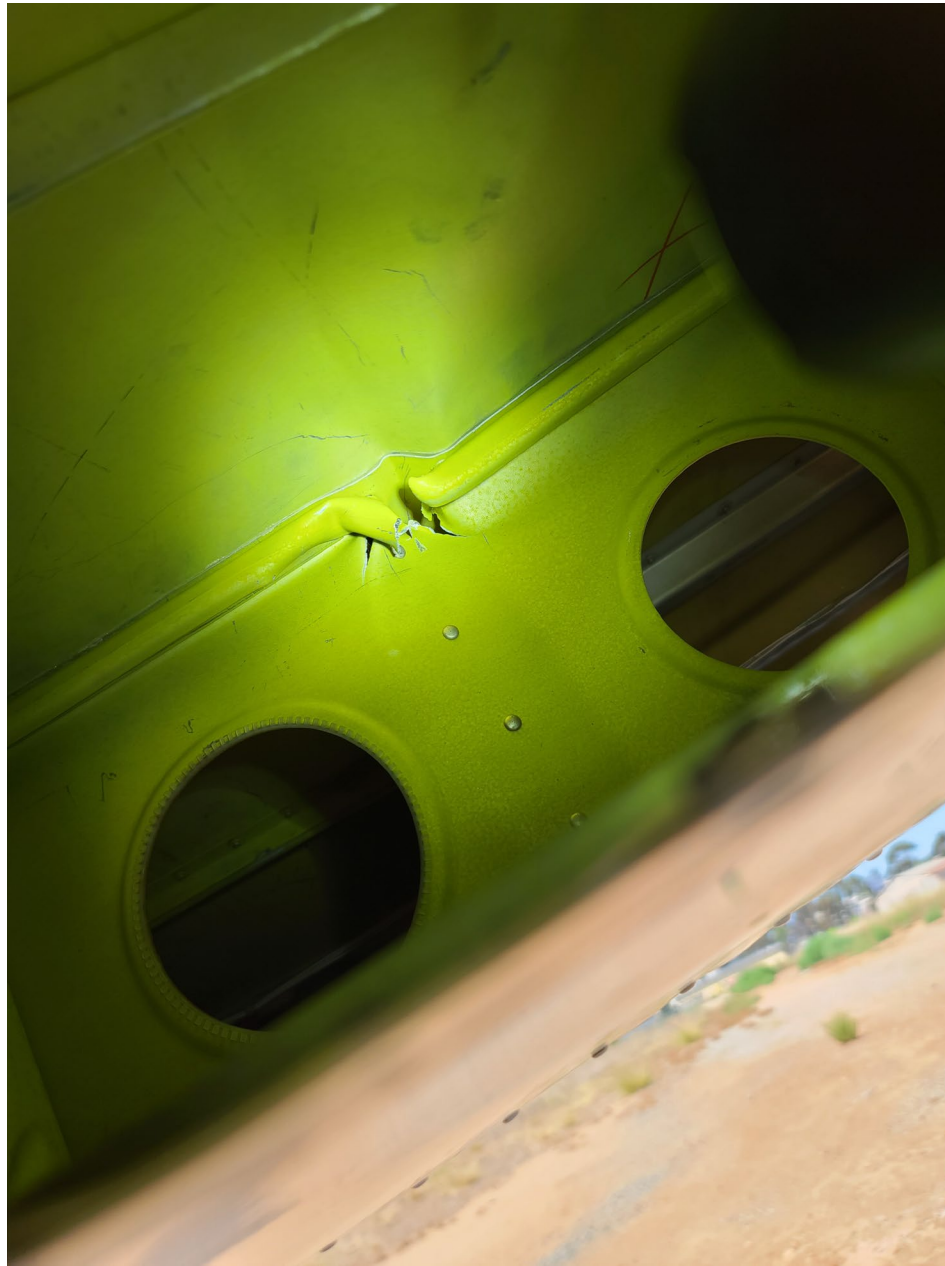
Photo 2 – View of damaged to the left-wing spar (courtesy of the FAA)
