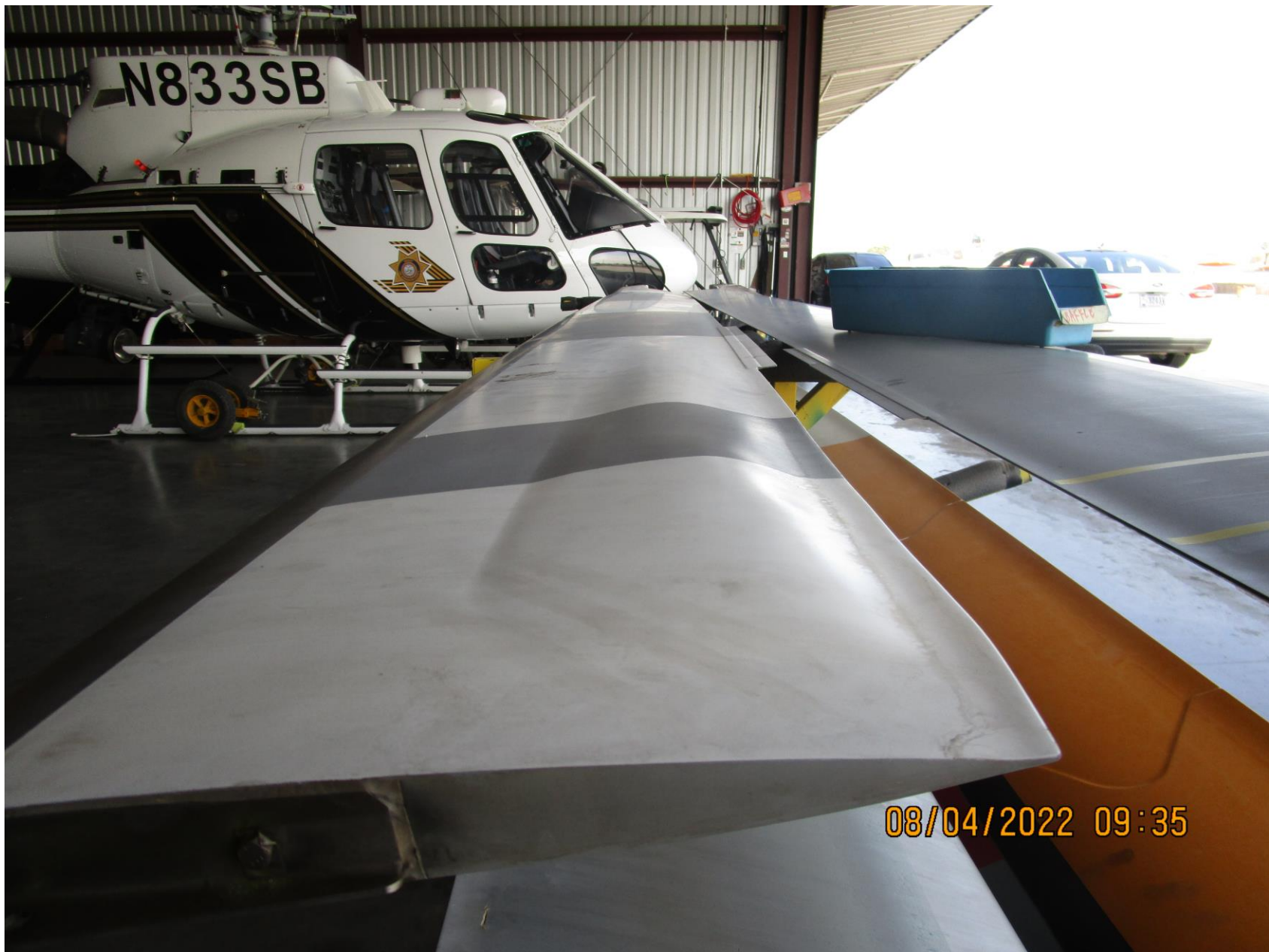
Photo 1 – Main rotor blade, delamination damage (Courtesy of the SBCSD).
