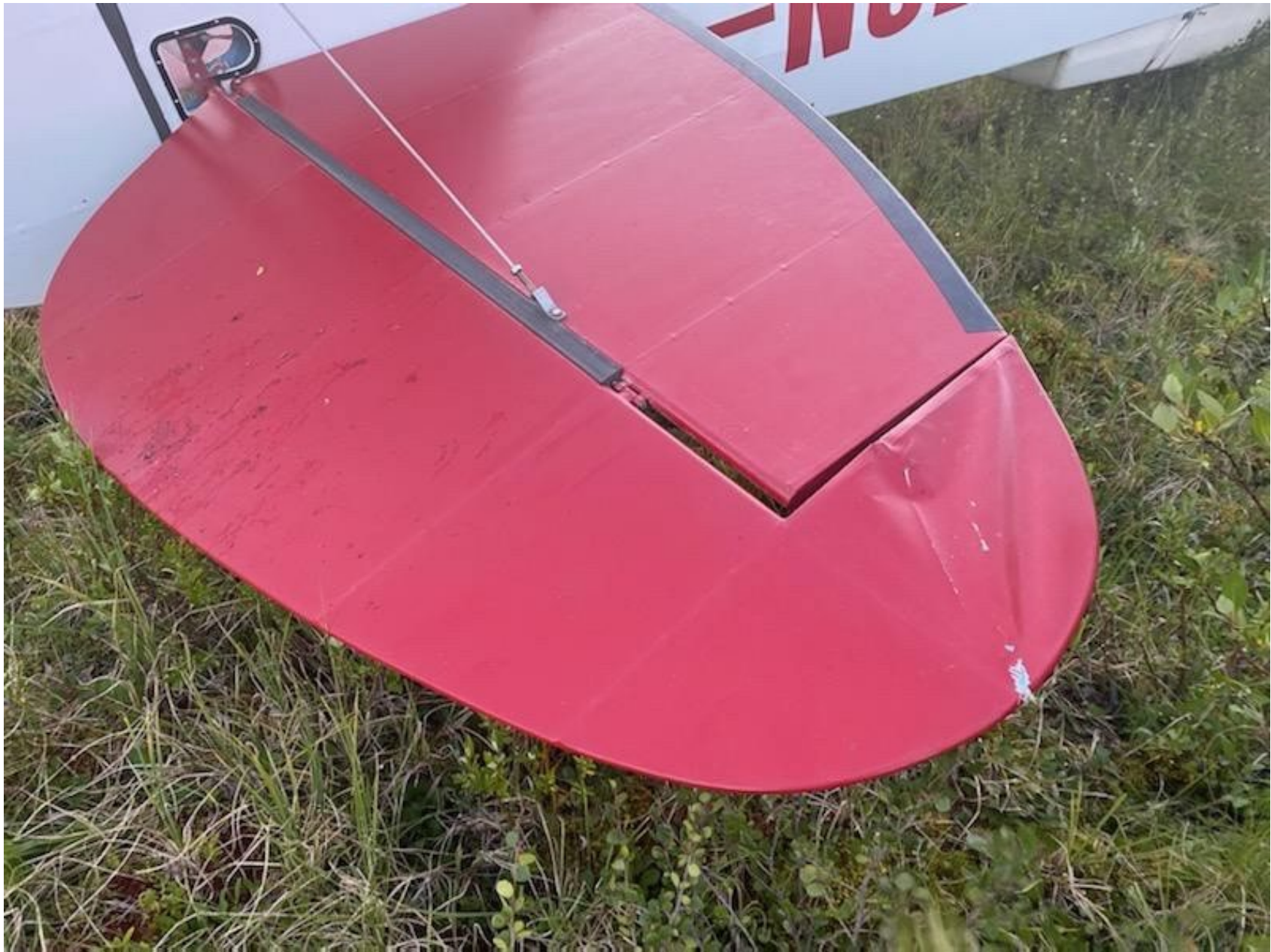
Photo 1 – View of leading-edge damage to right elevator (photo courtesy of operator)
