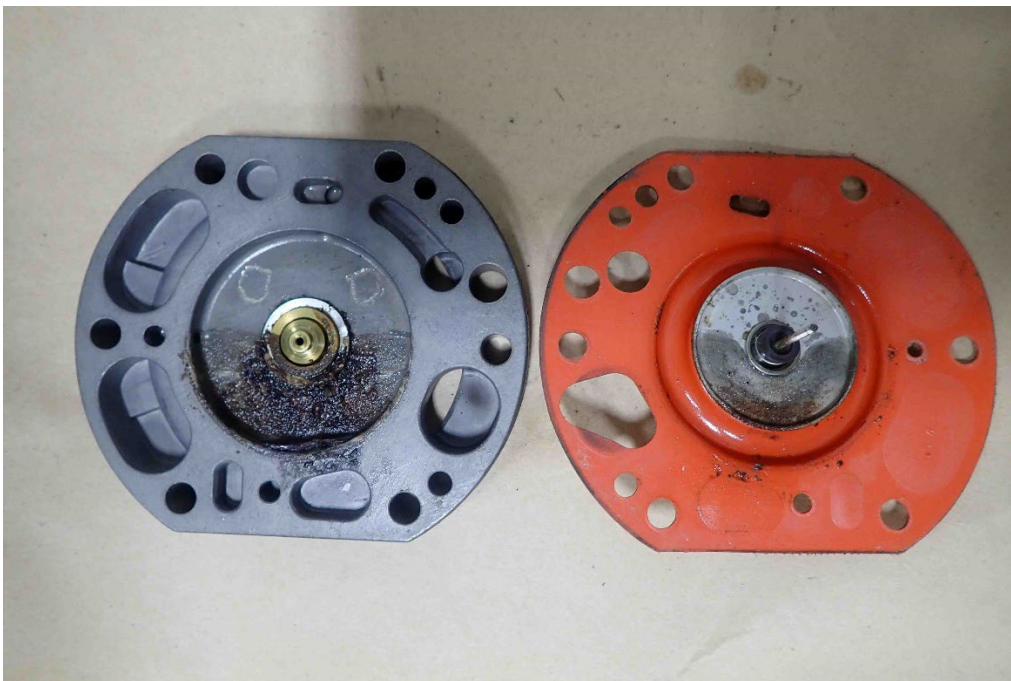
Figure 2 - Water line and corrosion on unmetered side
