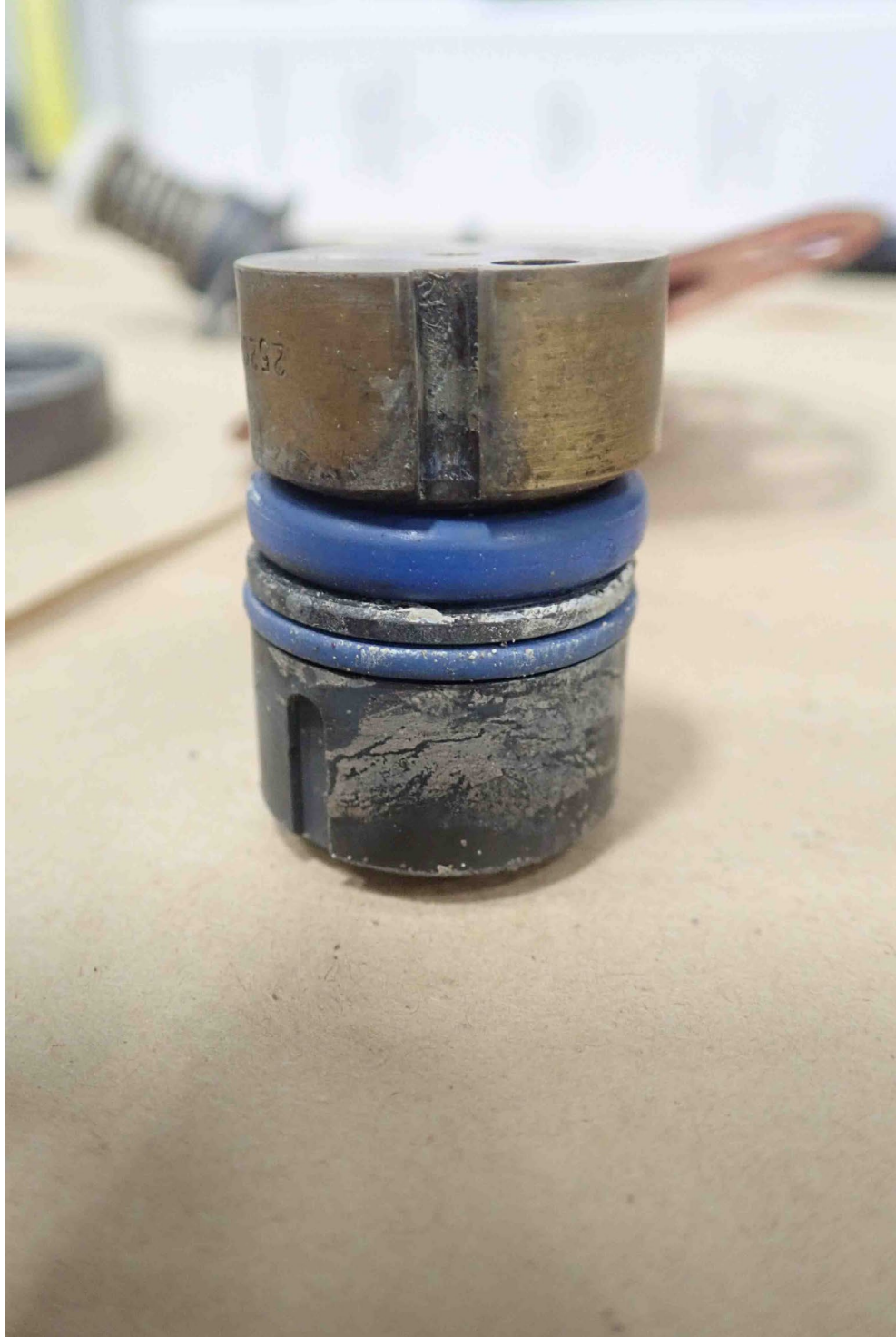
Figure 4 - Corrosion on the surfaces of the idle and mixture valve plugs
