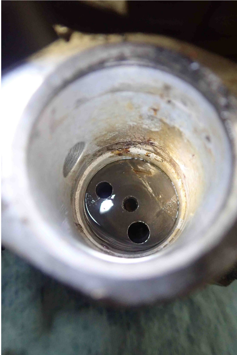
Figure 5 - Corrosion on the surfaces of the idle and mixture valve housing bore
