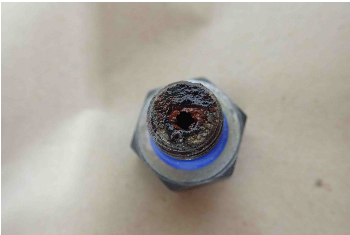
Figure 6 - Corrosion on alternate fuel outlet plug
