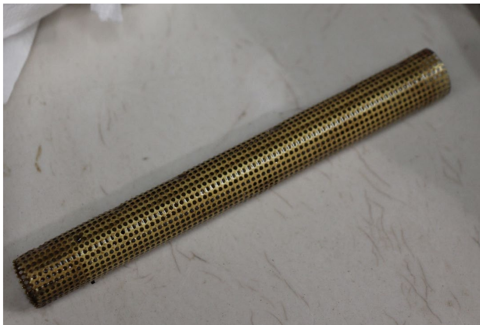
Photograph 7: Oil suction screen
