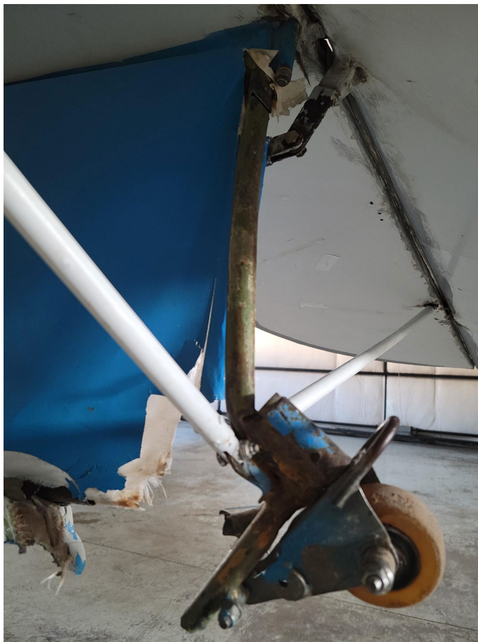
Photo 2 – Close up view of tailwheel damage (courtesy of the operator)
