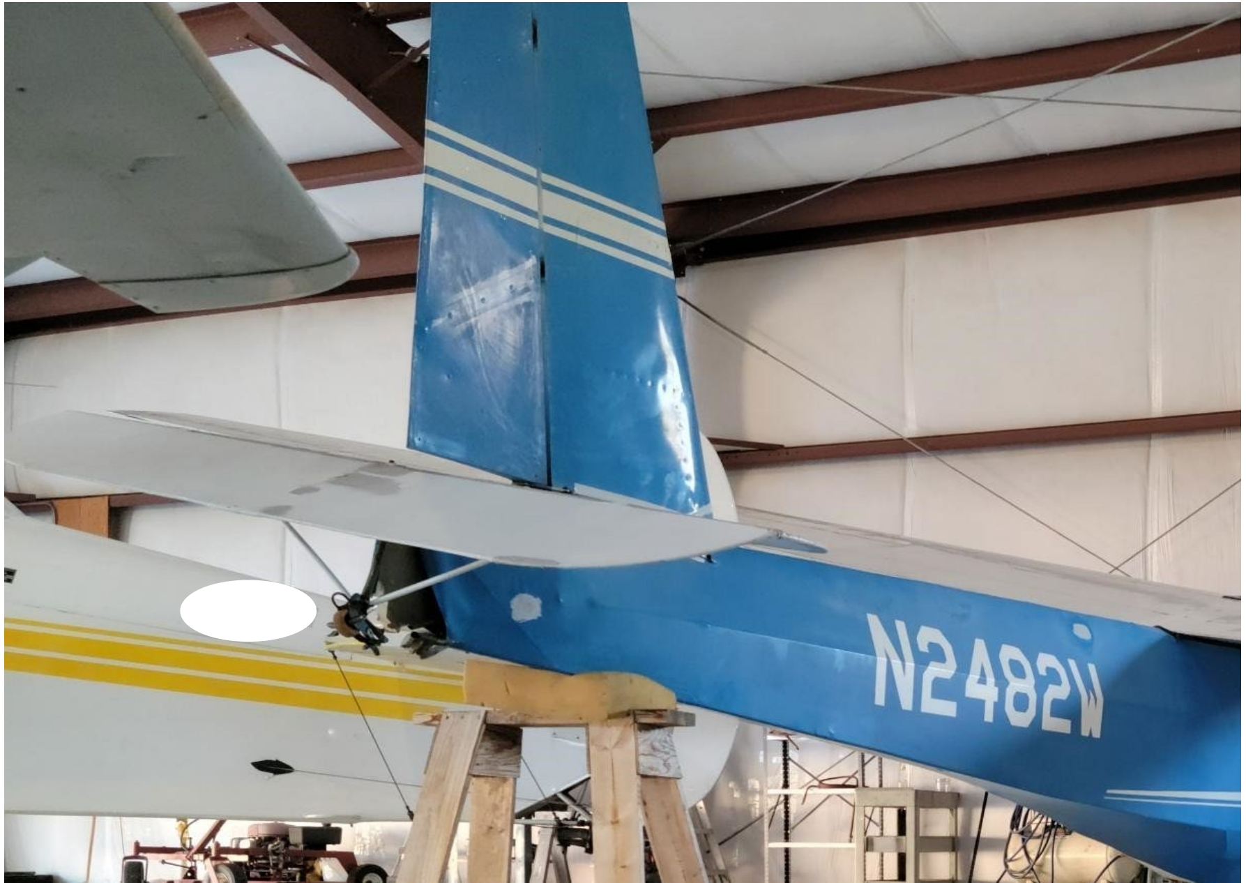
Photo 1 – View of empennage damage (courtesy of the operator)
