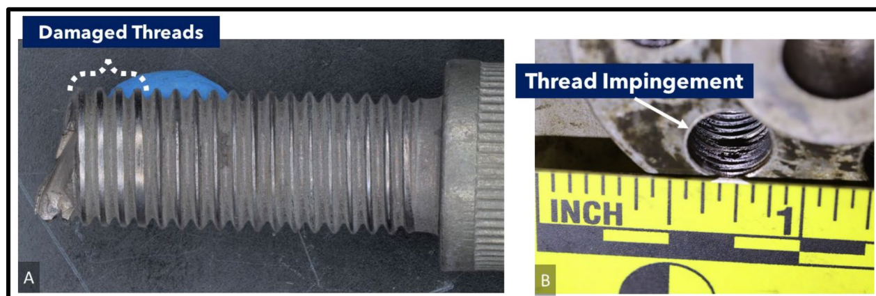
Figure 5: A Flywheel Screw with Damaged Threads, And Thread Imprints In The Corresponding Flywheel Hardware Hole)
