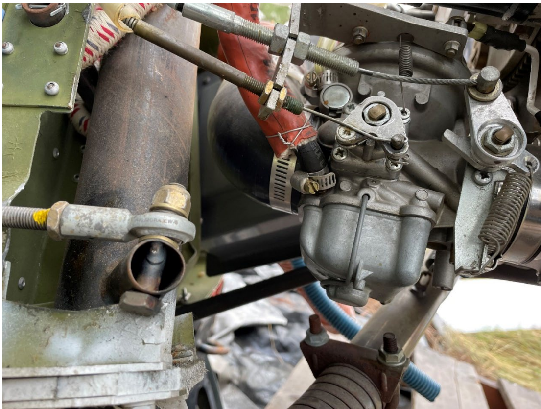
Figure 2. View of carburetor
