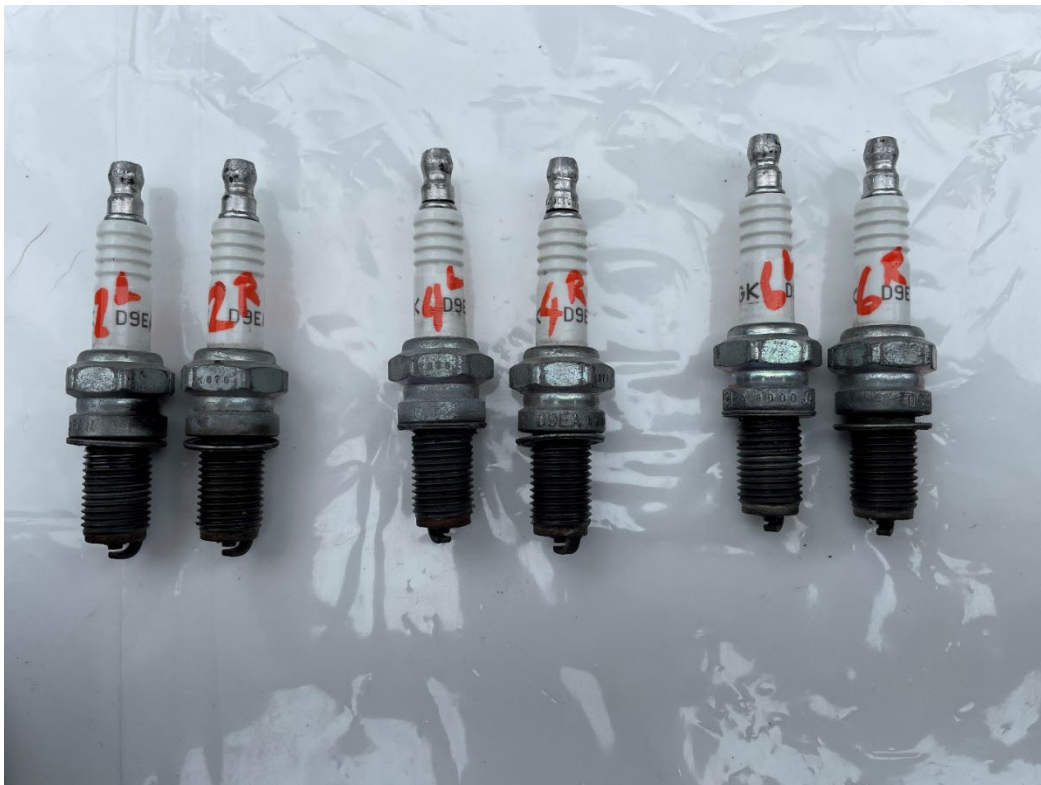
Figure 6. View of removed exhaust spark plugs
