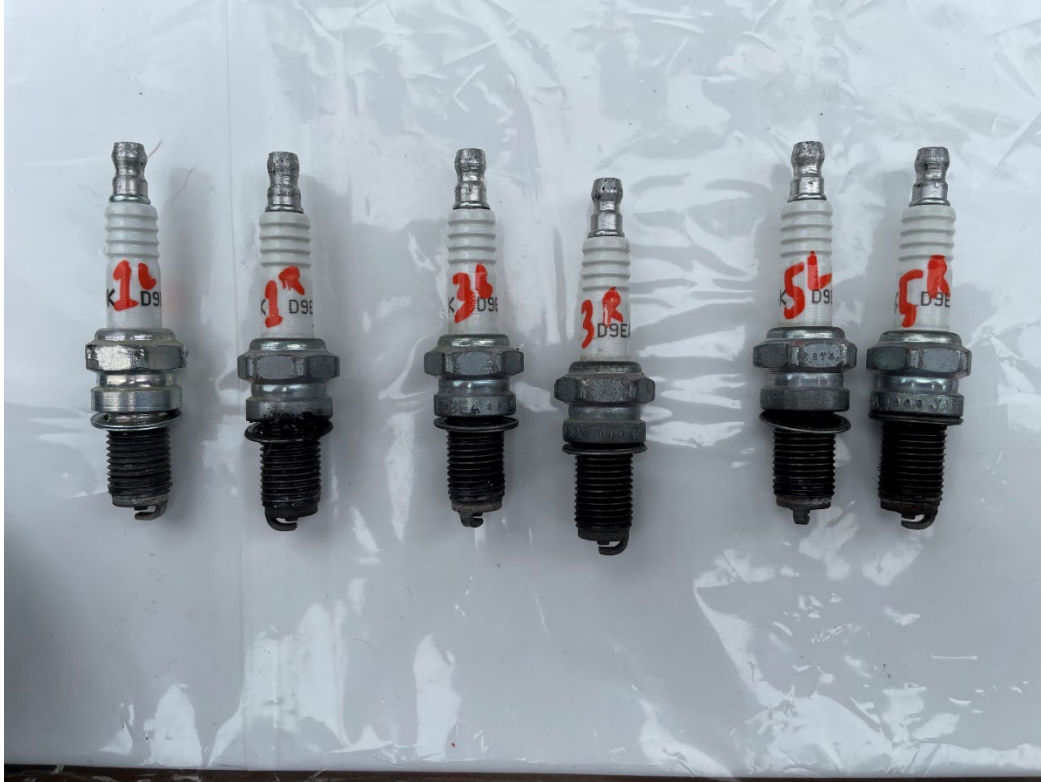
Figure 5. View of removed intake spark plugs
