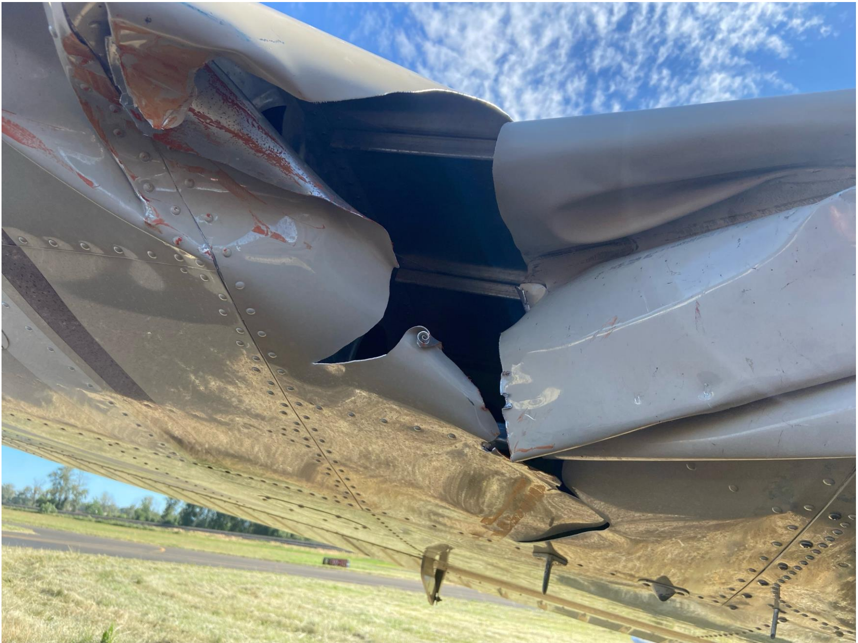
Photo 1 – Accident site, right wing damage. (Courtesy of the Owner)
