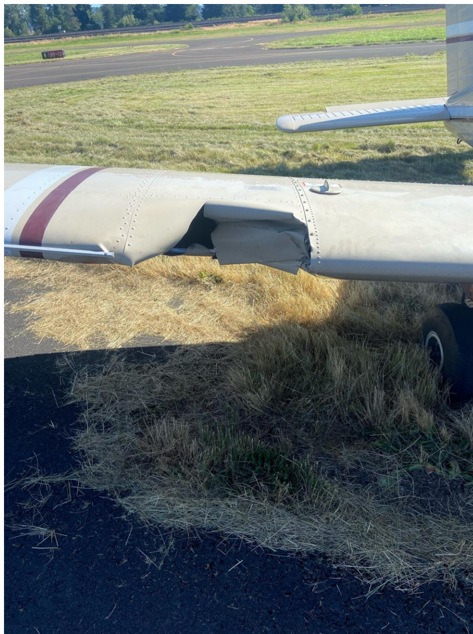
Photo 3 – Accident site, right wing damage. (Courtesy of the Owner)
