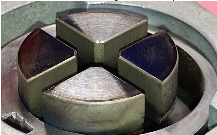
Photo #6 – Rotational scoring on the Rotor top surface
