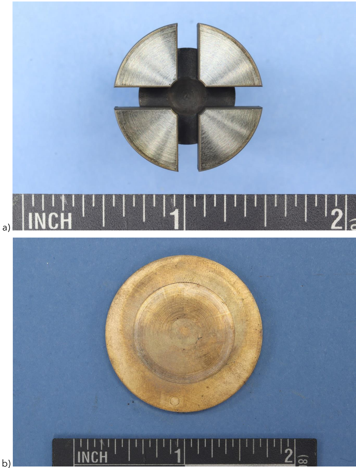
Figure 6. a) View of the rotor's drive end face and b) thrust plate against which the end face of the rotor rides.
