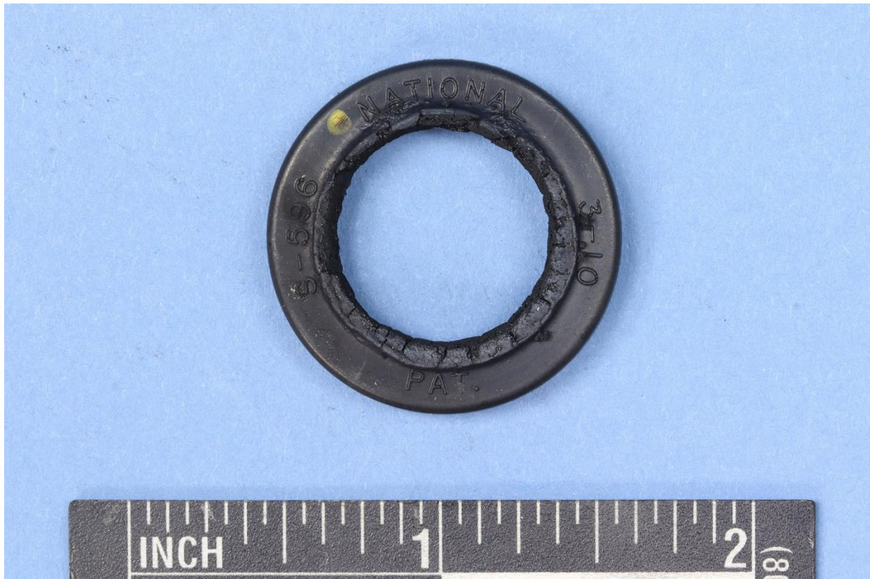
Figure 4. Image of the rubber seal that is installed on the driven end of the rotor showing thermal damage to the rubber.
