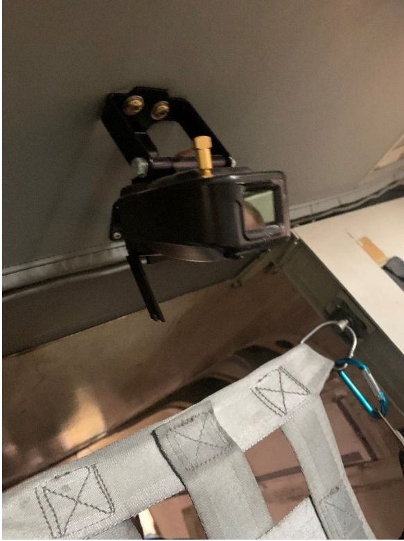
Figure 3: Appareo Camera as found in the Airplane.
