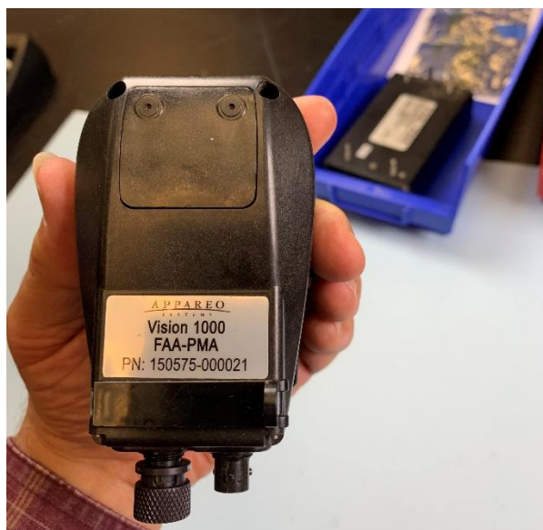
Figure 1. Photo of the Vision 1000 undamaged as received by the NTSB Vehicle Recorder Division.
