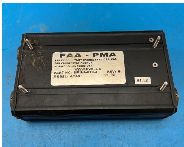
Figure 1. Photo of unit showing slight impact damage.
